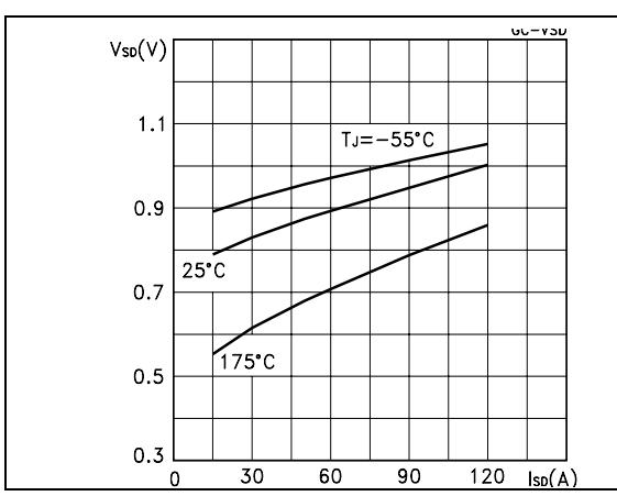
**Figure 12.** Source-drain diode forward characteristics
