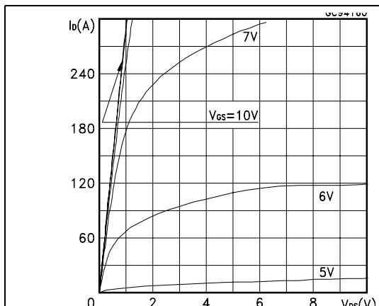
Figure 4. Transfer characteristics
