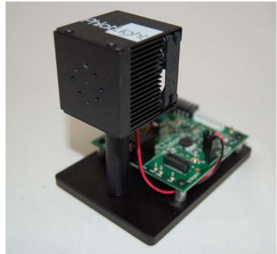
Figure 2: Heat sink / Driver board Assembly
