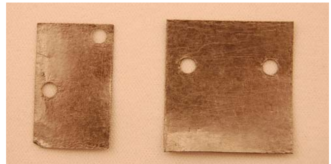
Figure 5: Left picture: TIM cut for C21 package types. Right picture: TIM cut for C11 package types.
