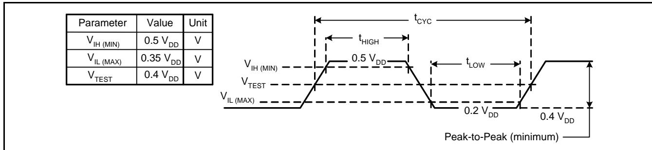
Figure 4. Clock Waveform
