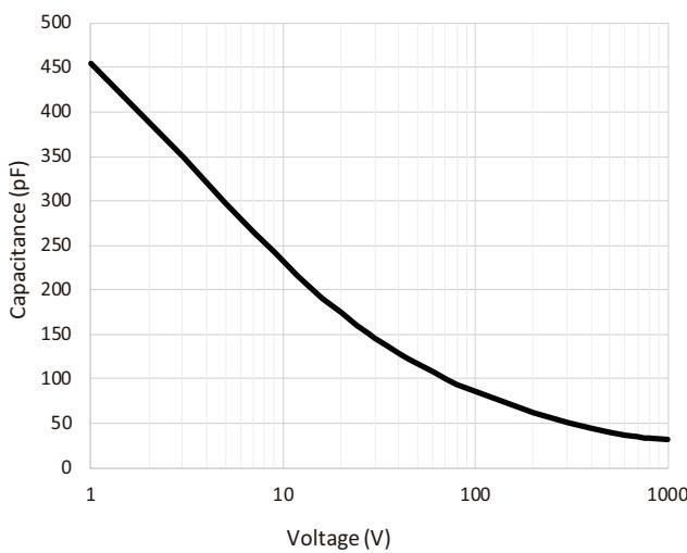
**Figure 6: Capacitive Charge vs. Reverse Voltage (Per Leg)**
