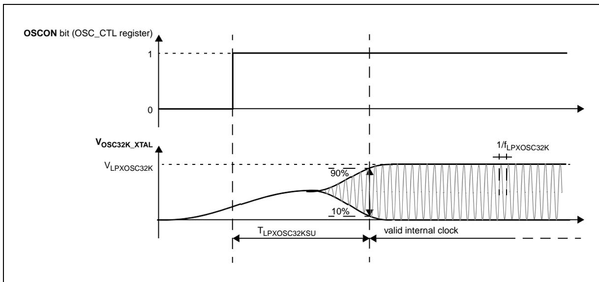
Figure 14. Slow external crystal oscillator (32 kHz) electrical characteristics
