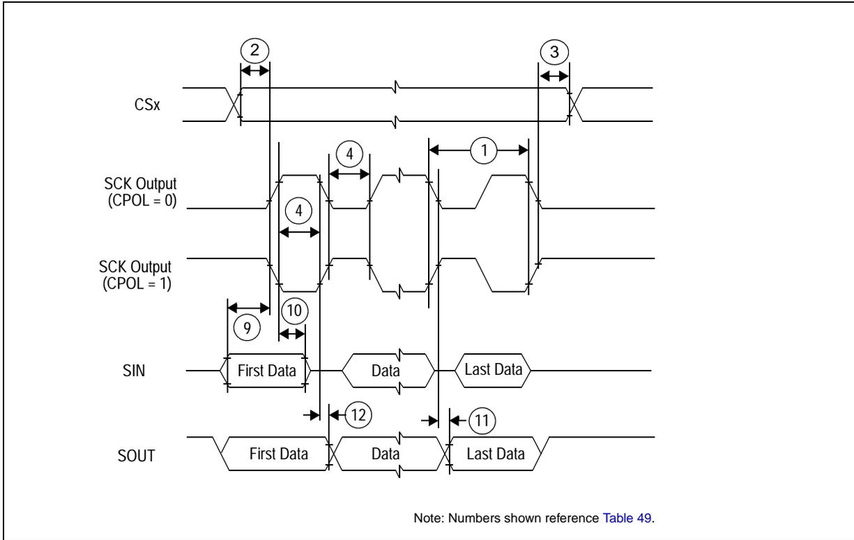
**Figure 25. DSPI classic SPI timing—master, CPHA = 0**
