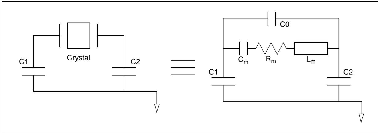
Figure 13. Equivalent circuit of a quartz crystal
