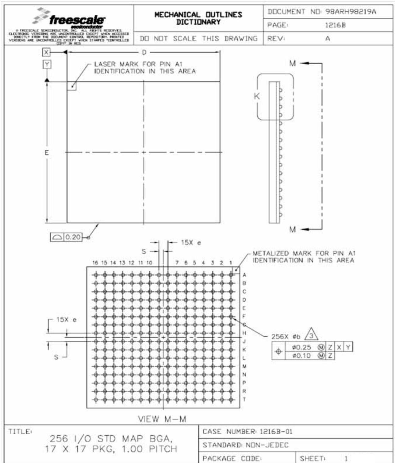
Figure 43. 256 MAPBGA mechanical drawing (Part 1 of 2)
