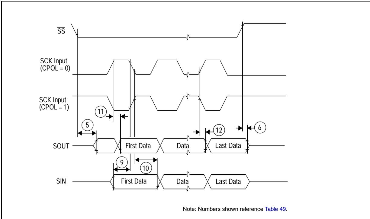
Figure 32. DSPI modified transfer format timing–slave, CPHA = 1
