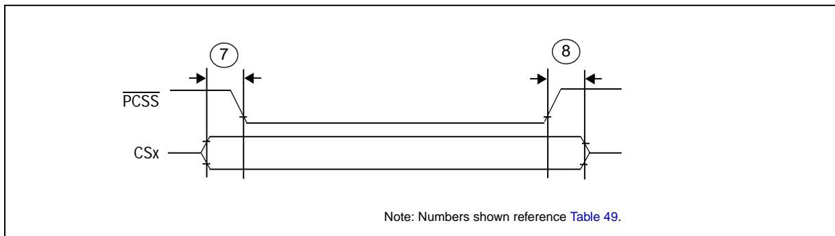
Figure 33. DSPI PCS strobe ( $\overline{\text{PCSS}}$ ) timing
