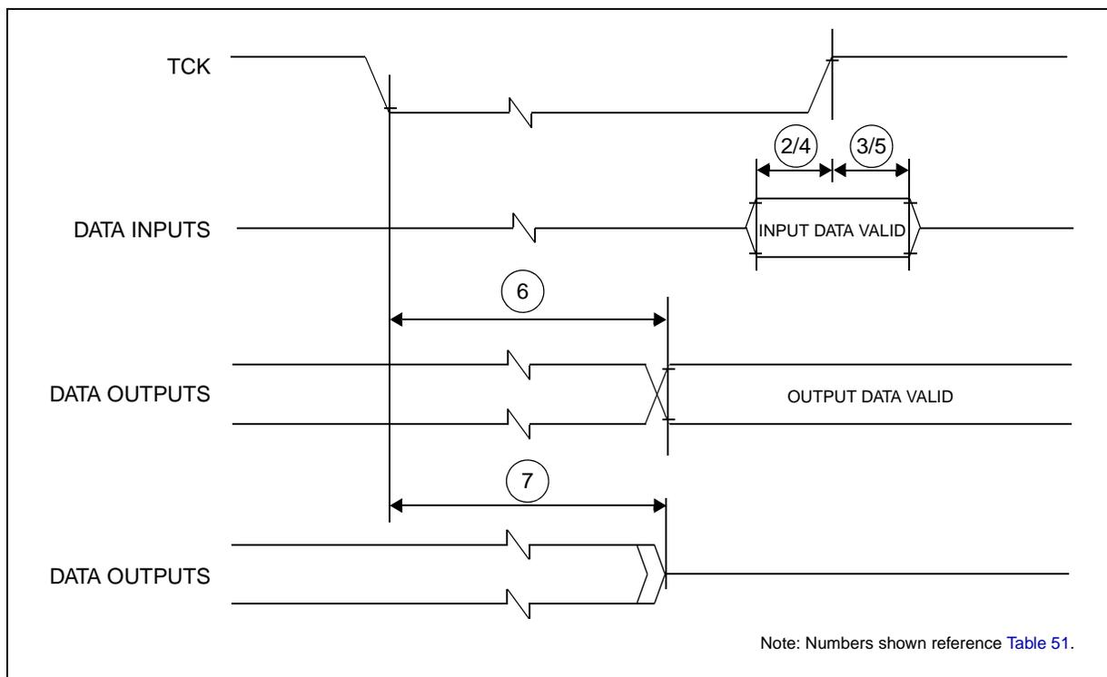
Figure 36. Timing diagram - JTAG boundary scan
