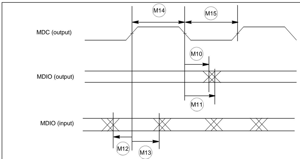
Figure 24. MII serial management channel timing diagram
