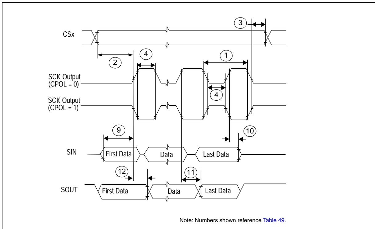
**Figure 29. DSPI modified transfer format timing—master, CPHA = 0**
