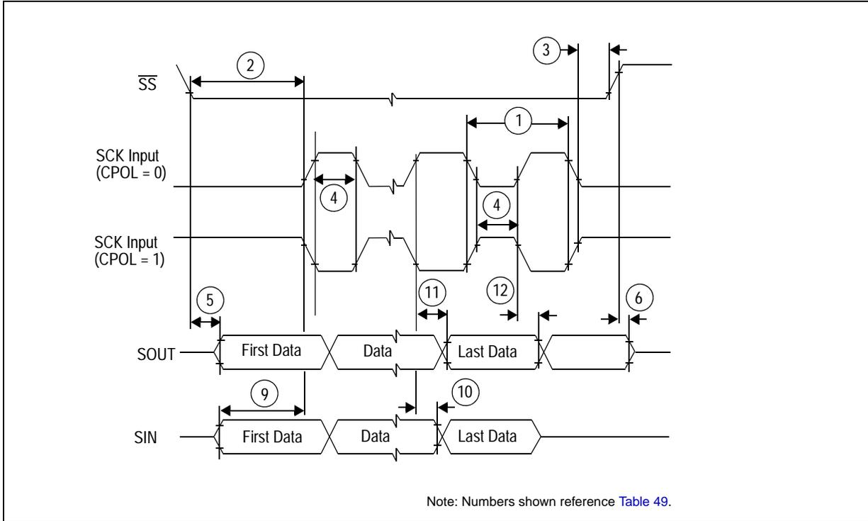
Figure 31. DSPI modified transfer format timing–slave, CPHA = 0
