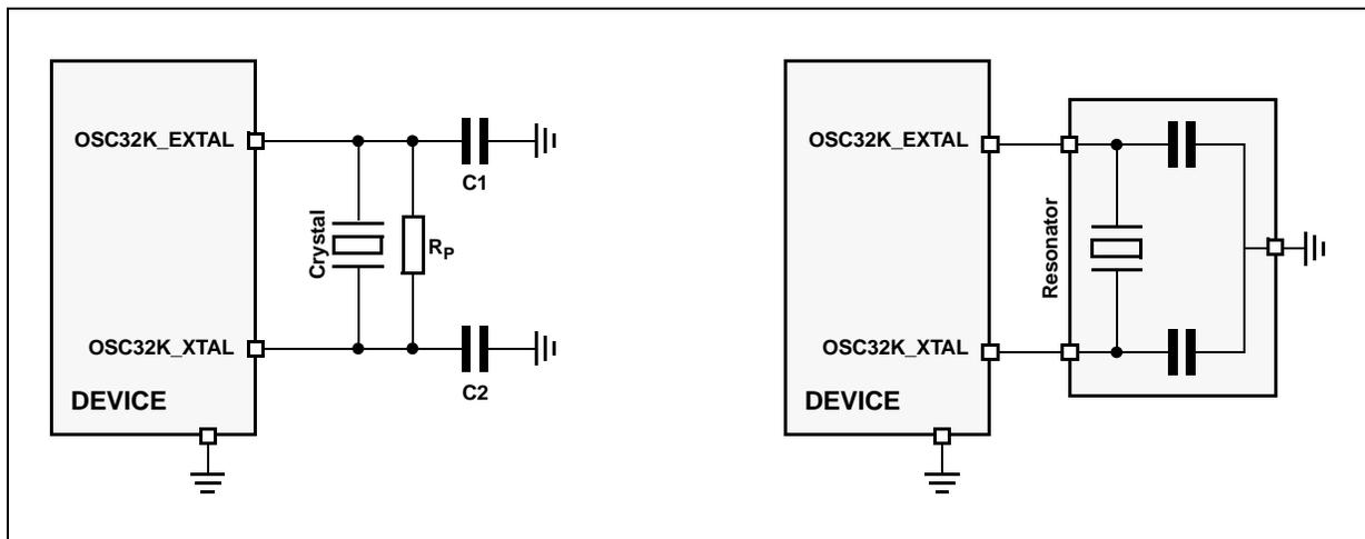
**Figure 12. Crystal oscillator and resonator connection scheme**
