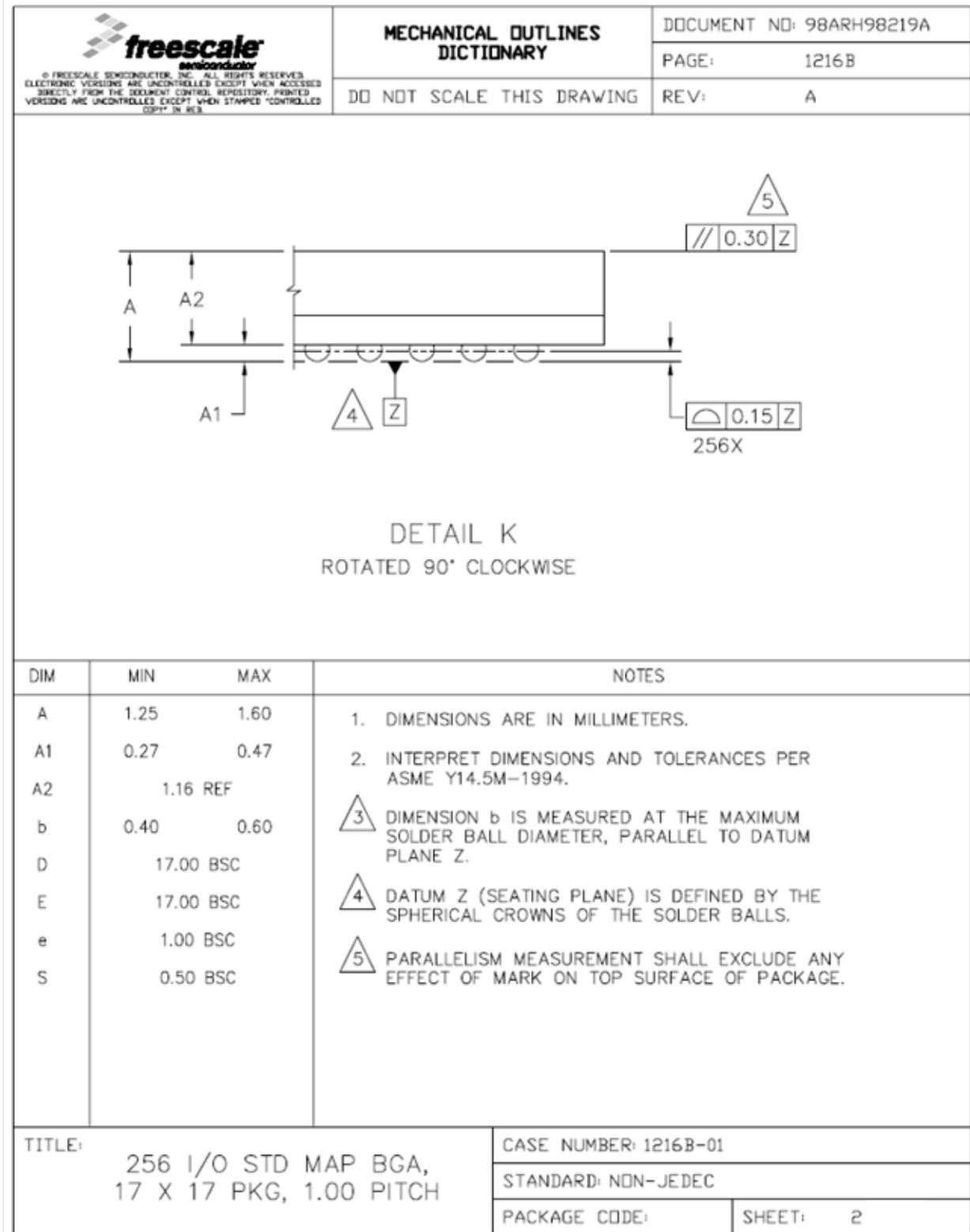
Figure 44. 256 MAPBGA mechanical drawing (Part 2 of 2)
