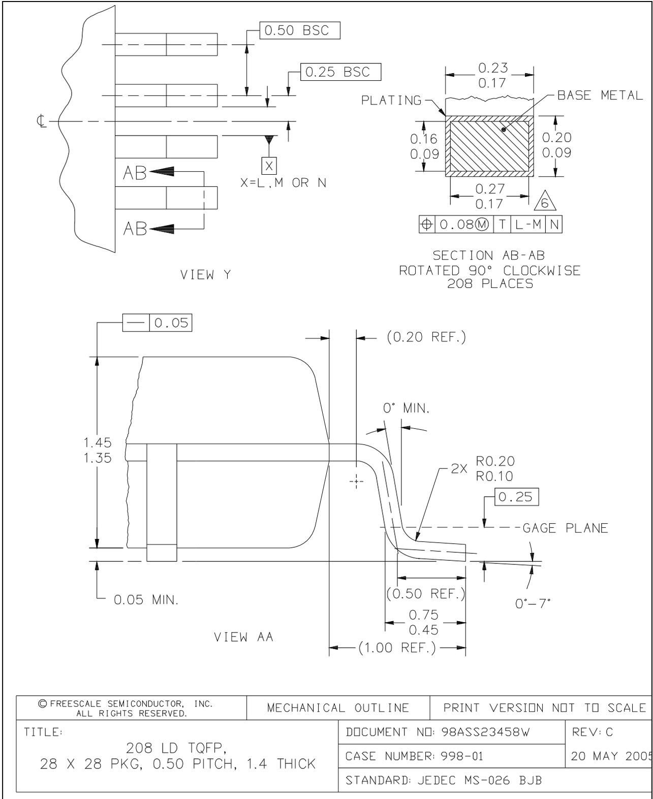
Figure 41. 208 LQFP mechanical drawing (Part 2 of 3)
