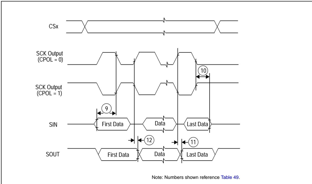
**Figure 26. DSPI classic SPI timing—master, CPHA = 1**
