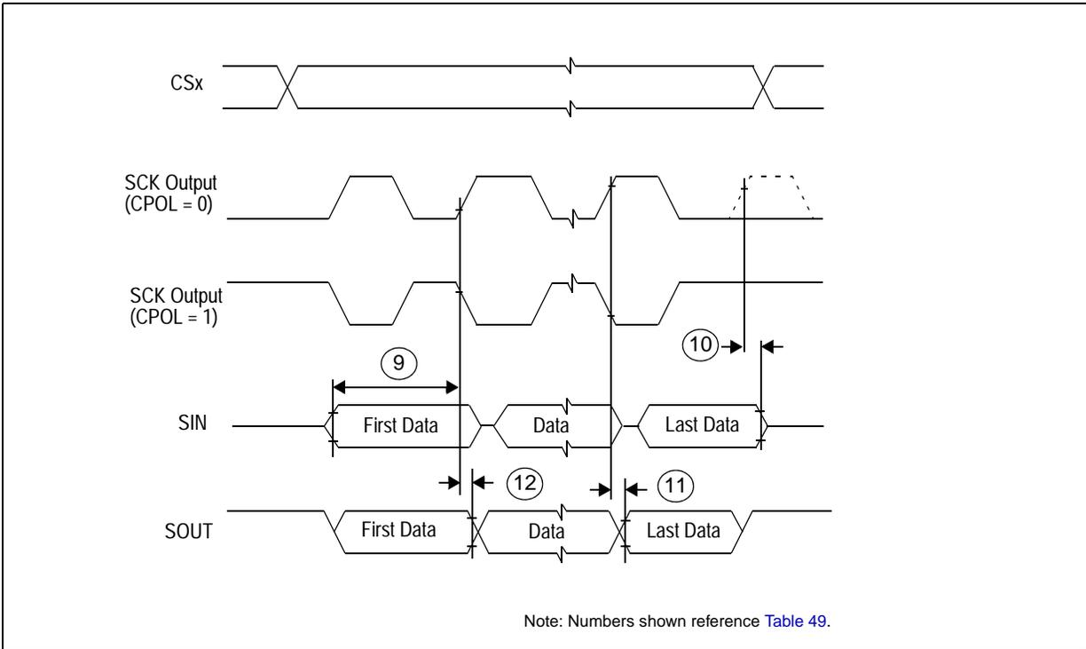
Figure 30. DSPI modified transfer format timing—master, CPHA = 1
