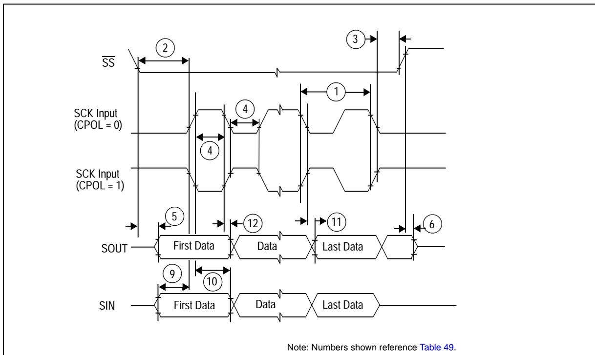
Figure 27. DSPI classic SPI timing—slave, CPHA = 0
