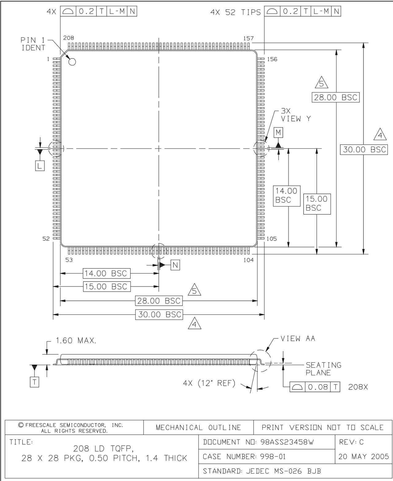
Figure 40. 208 LQFP mechanical drawing (Part 1 of 3)
