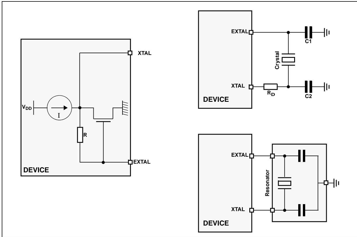
Figure 10. Crystal oscillator and resonator connection scheme
