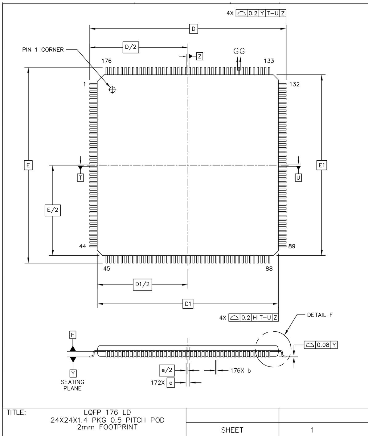
Figure 37. 176 LQFP mechanical drawing (Part 1 of 3)
