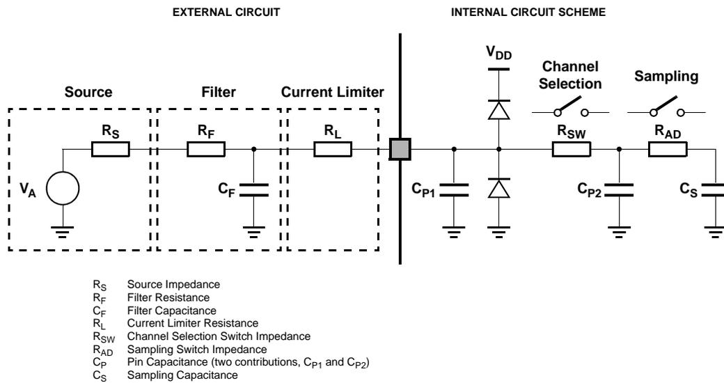
**Figure 16. Input equivalent circuit (precise channels)**
