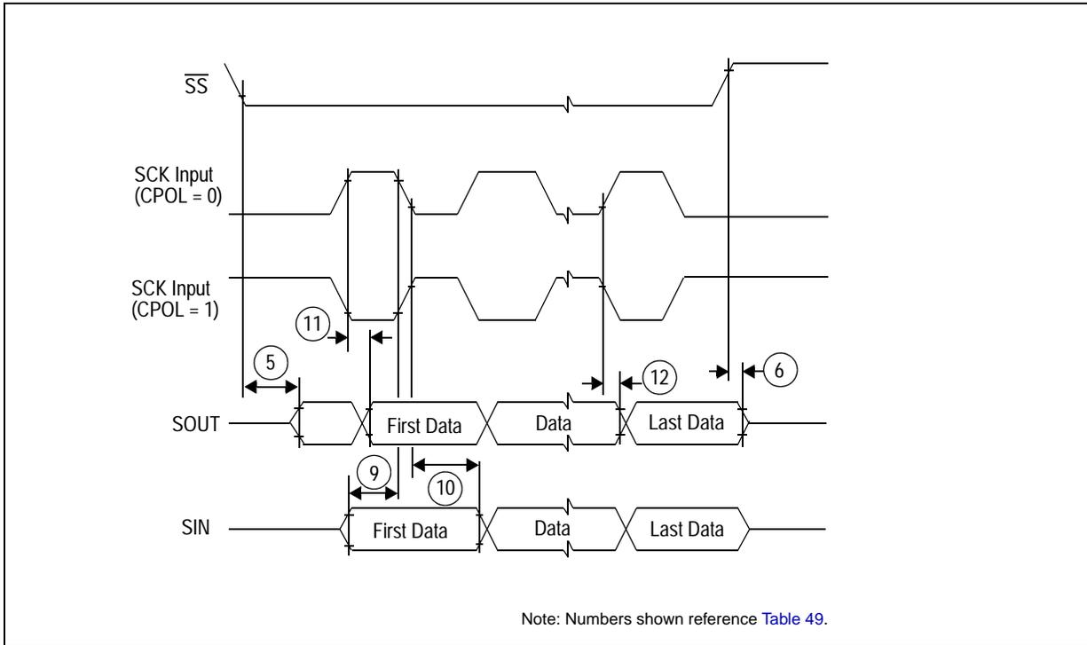
**Figure 28. DSPI classic SPI timing—slave, CPHA = 1**
