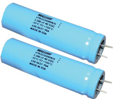
Type VPR is a radial leaded aluminum electrolytic capacitor with a 105 °C, 2000 hours long life ratings. The VPR has 3 optional case styles with a third lead. The low ESR rating makes it ideal for output filtering in switching power supplies.
