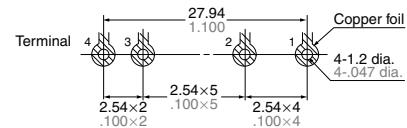
Tolerance:  $\pm 0.1 \pm .004$ General tolerance:  $\pm 0.5 \pm .020$
