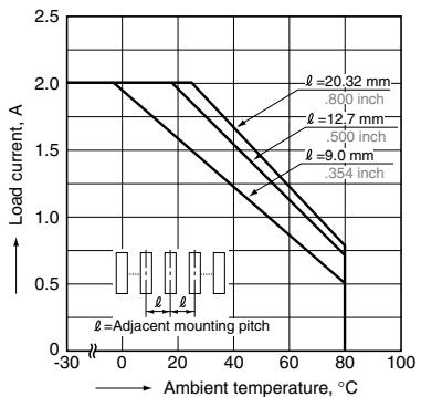
4.- (2) Characteristics of load current vs. ambient temperature for adjacent mounting
