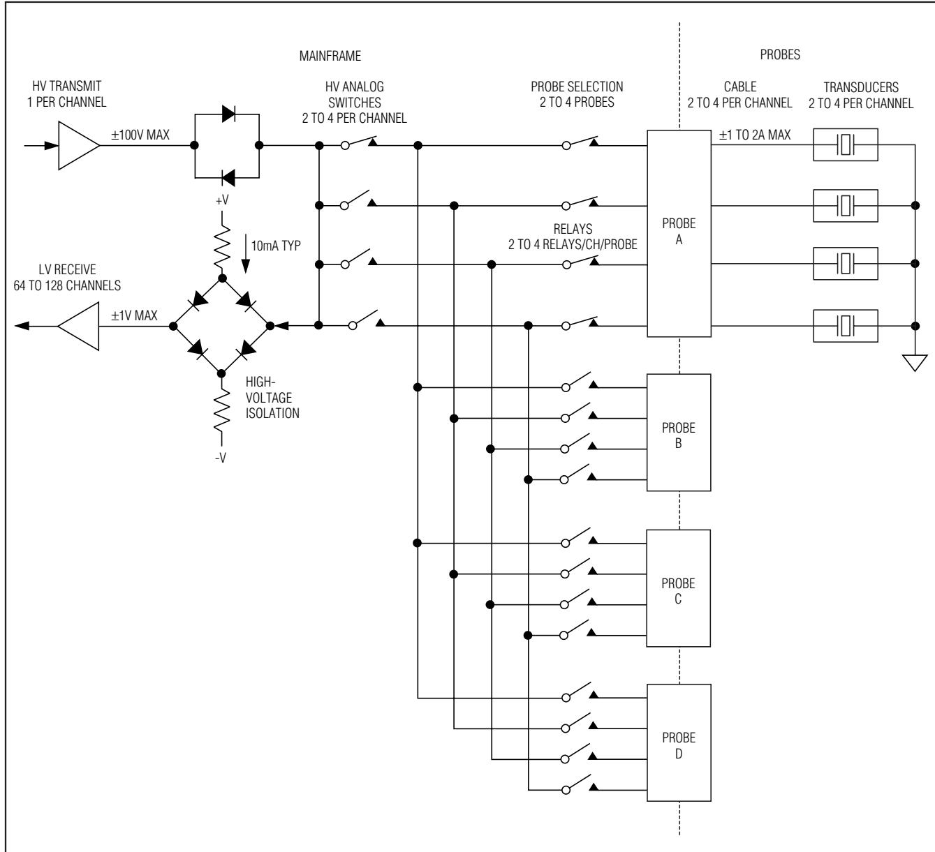
Figure 5. Medical Ultrasound Application—High-Voltage Analog Switches in Mainframe
