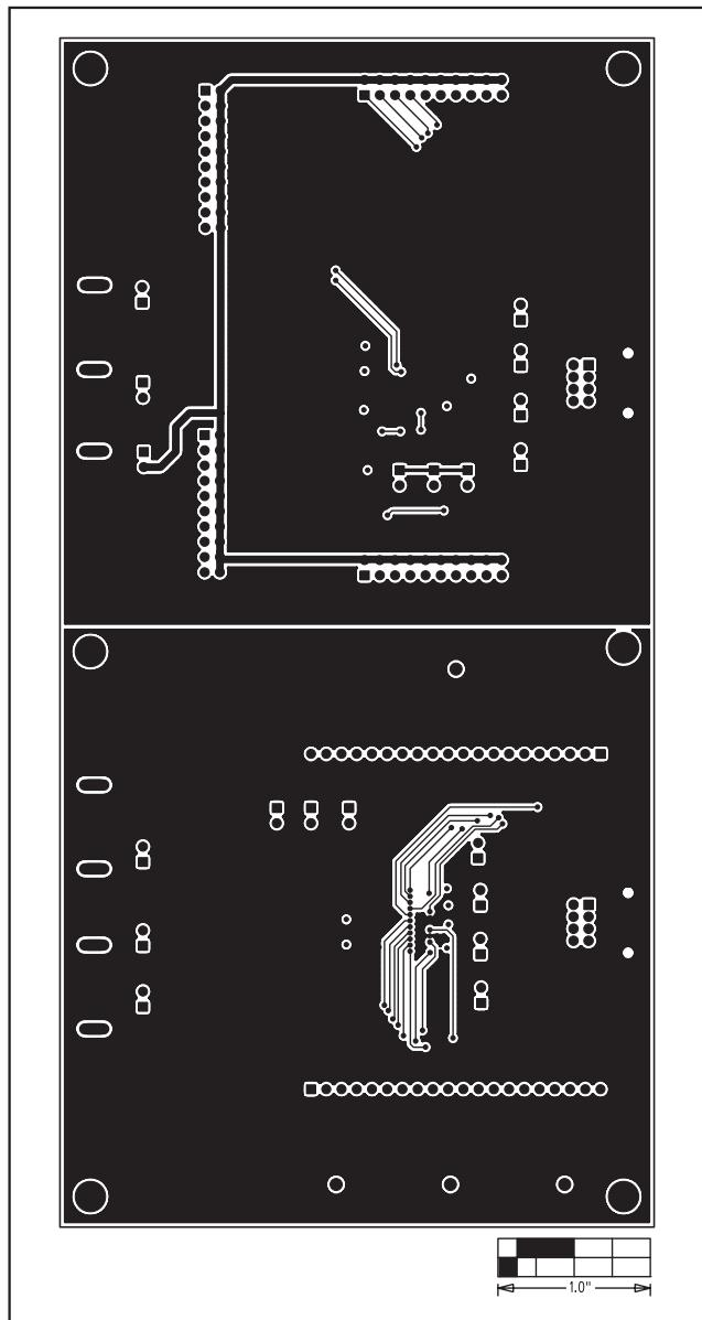
Figure 6. MAX9209/MAX9244 EV Kit PCB Layout—Solder Side
