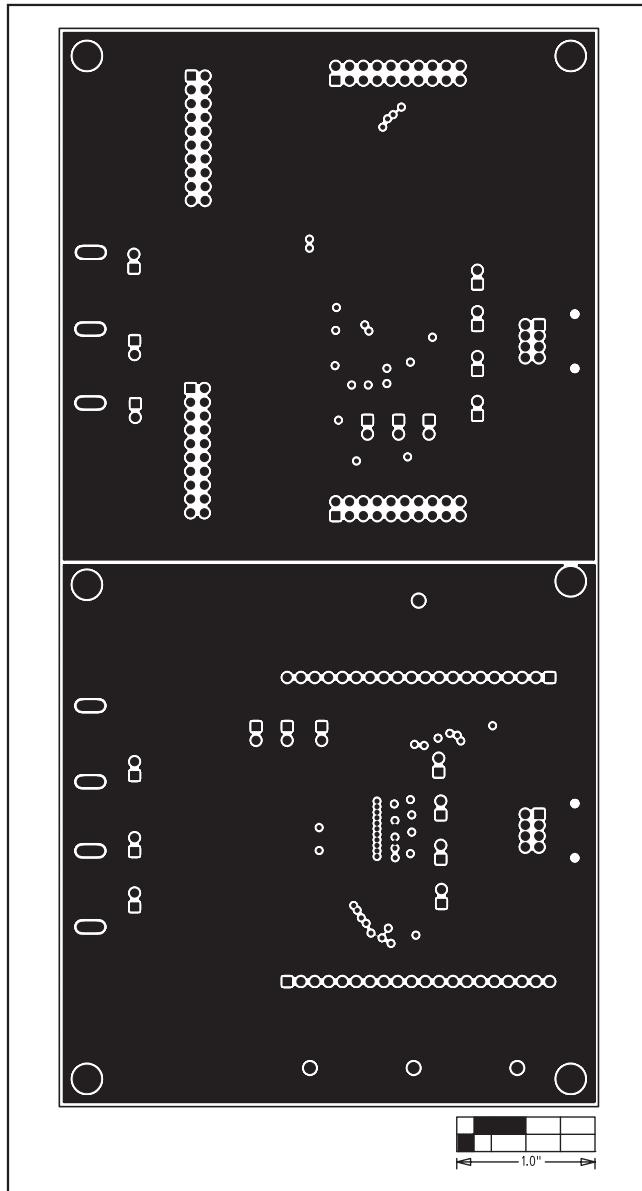
Figure 4. MAX9209/MAX9244 EV Kit PCB Layout—Inner Layer 2
