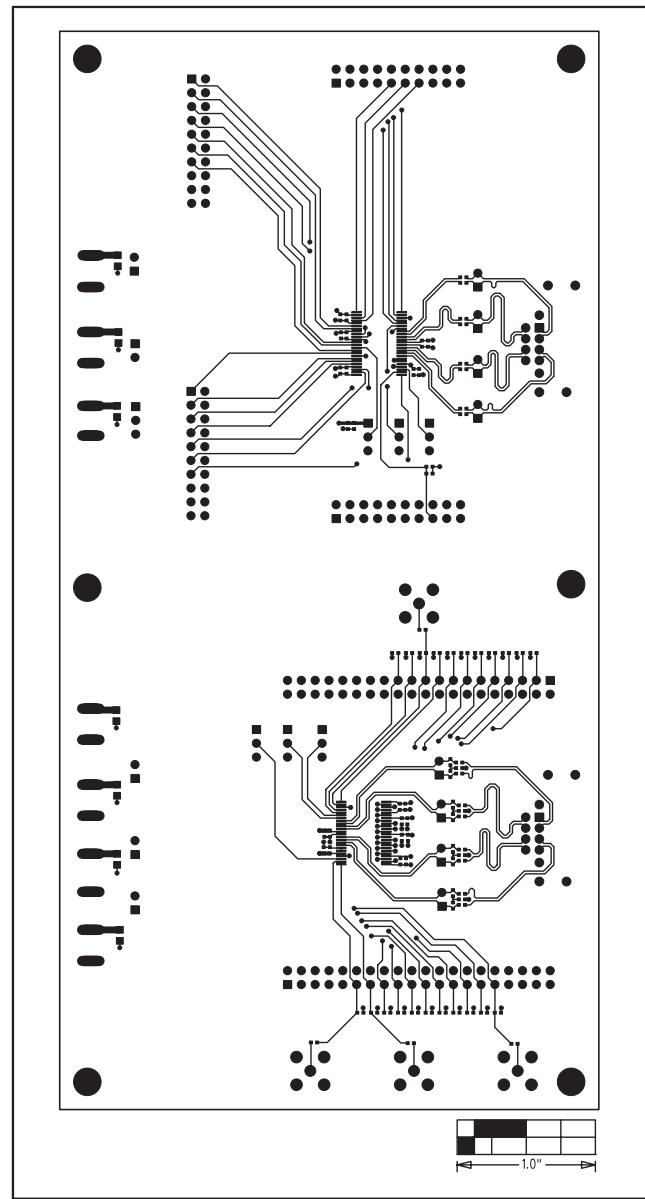
Figure 3. MAX9209/MAX9244 EV Kit PCB Layout—Component Side
