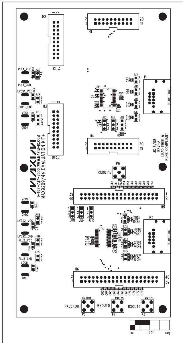
Figure 2. MAX9209/MAX9244 EV Kit Component Placement Guide—Component Side
