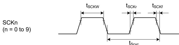
Figure 2.37 SCI clock input/output timing
