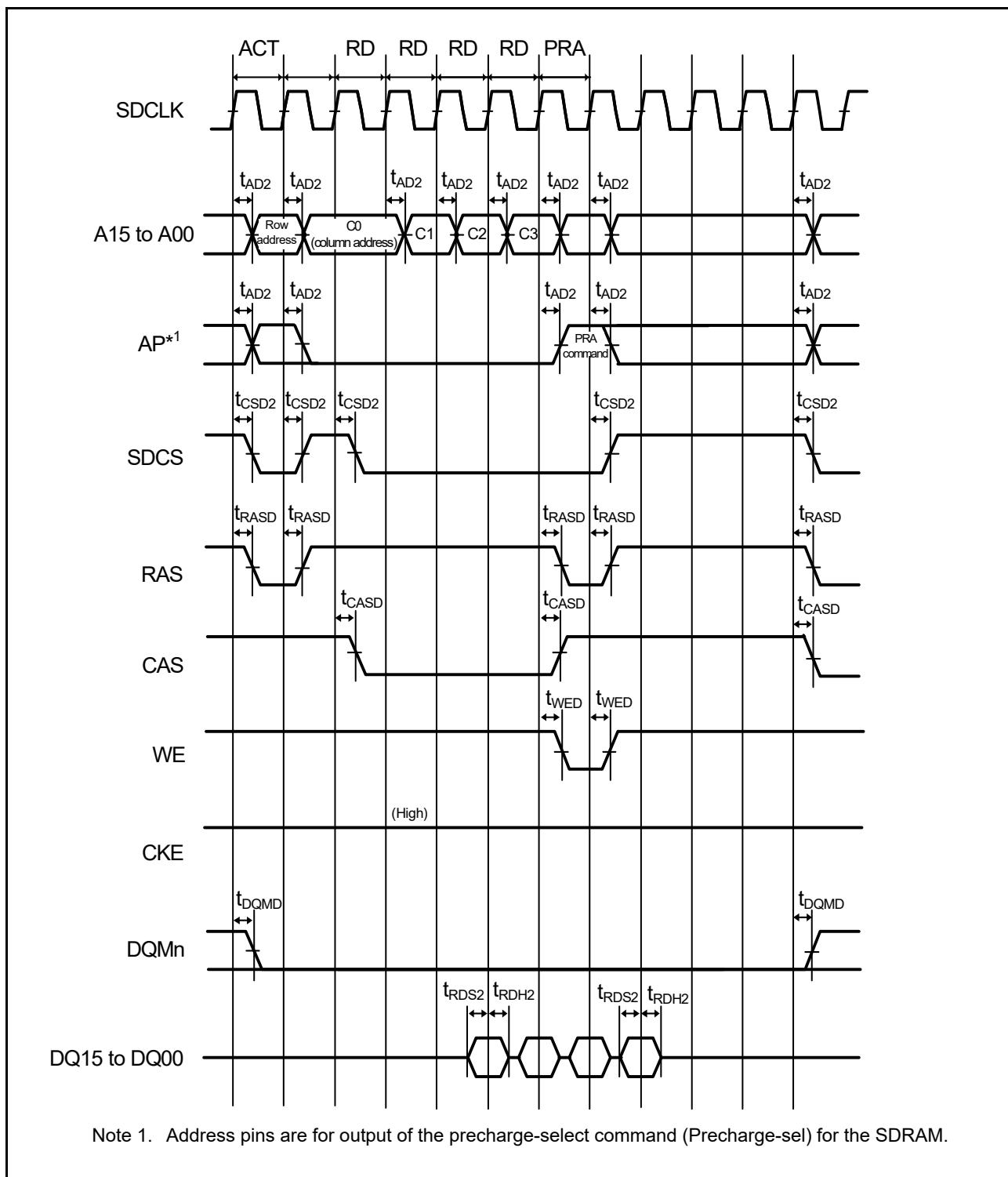
Figure 2.23 SDRAM multiple read timing
