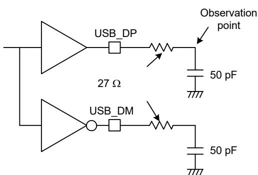
**Figure 2.87 Test circuit in full-speed mode**
