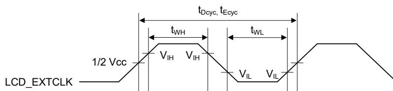
**Figure 2.73 LCD\_EXTCLK clock input timing**
