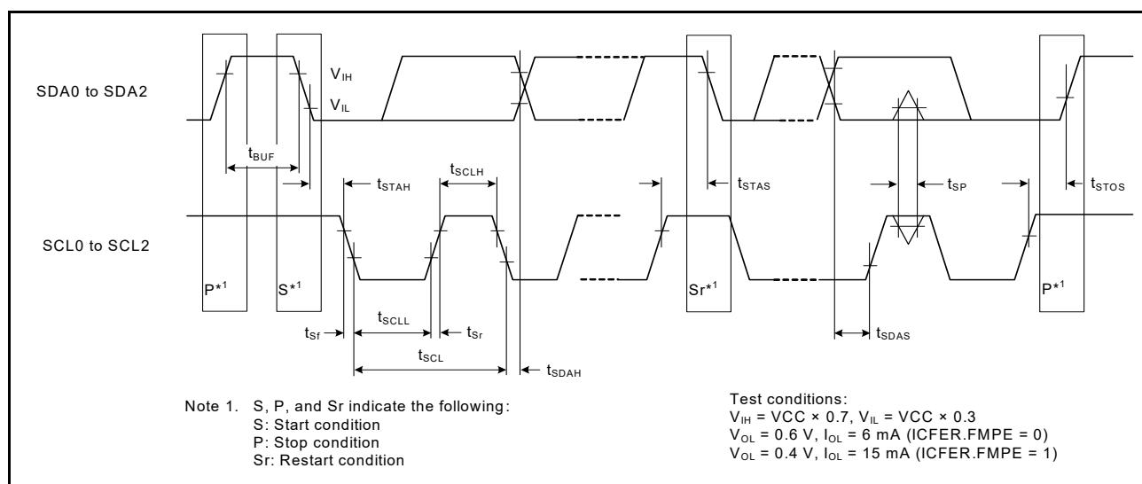
**Figure 2.54 I<sup>2</sup>C bus interface input/output timing**
