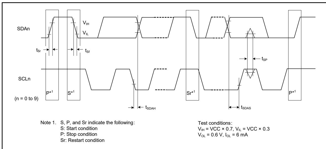
Figure 2.44 SCI simple IIC mode timing
