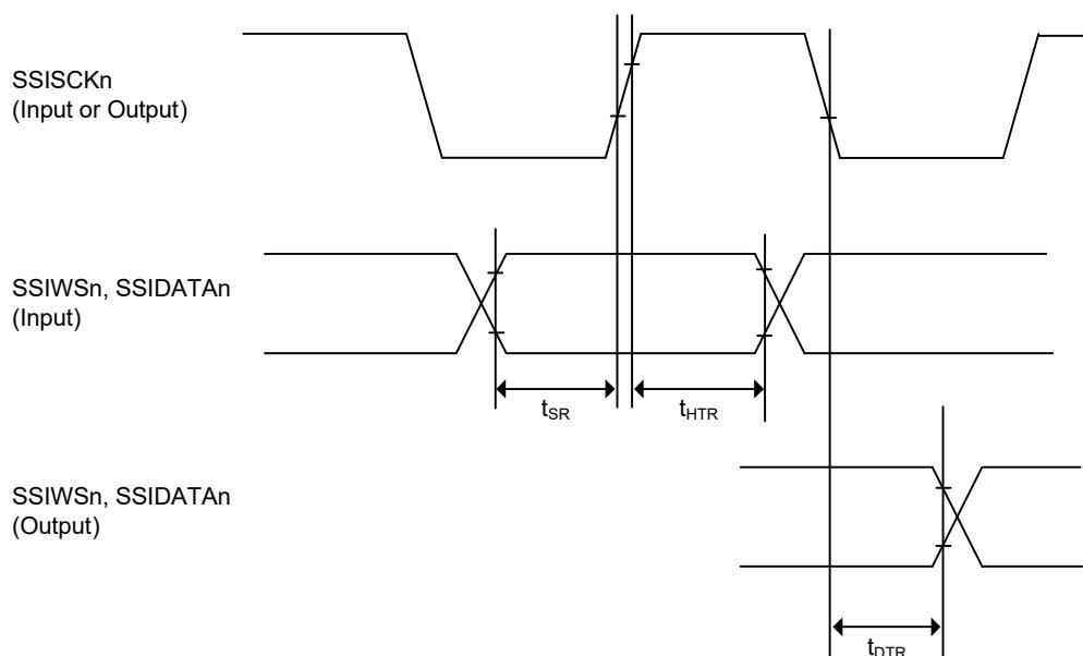
**Figure 2.56 SSI data transmit and receive timing when SSICR.SCKP = 0**
