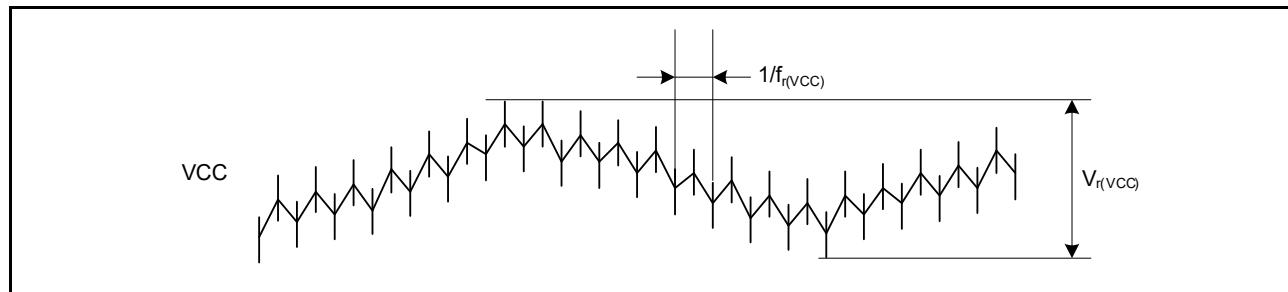
**Figure 2.2 Ripple waveform**
