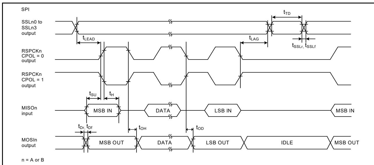
Figure 2.46 SPI timing for master when CPHA = 0
