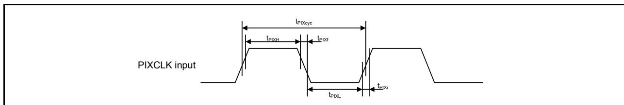
**Figure 2.70 PDC input clock timing**
