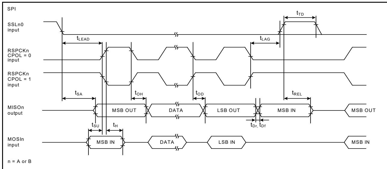
**Figure 2.50 SPI timing for slave when  $\text{CPHA} = 0$**
