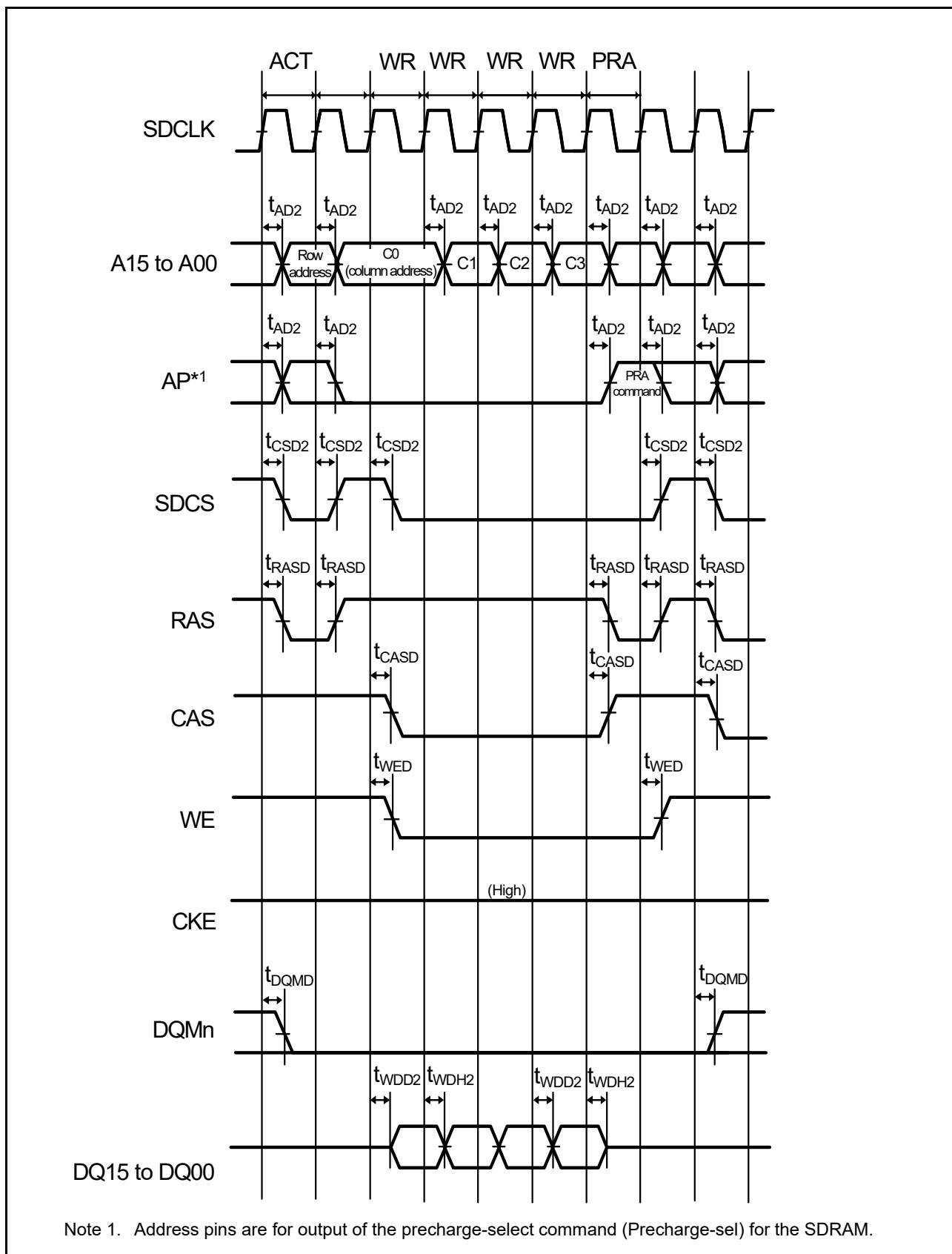
Figure 2.24 SDRAM multiple write timing
