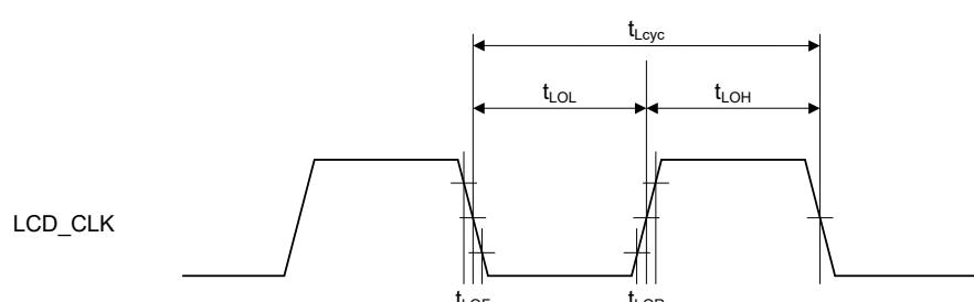
**Figure 2.74 LCD\_CLK clock output timing**
