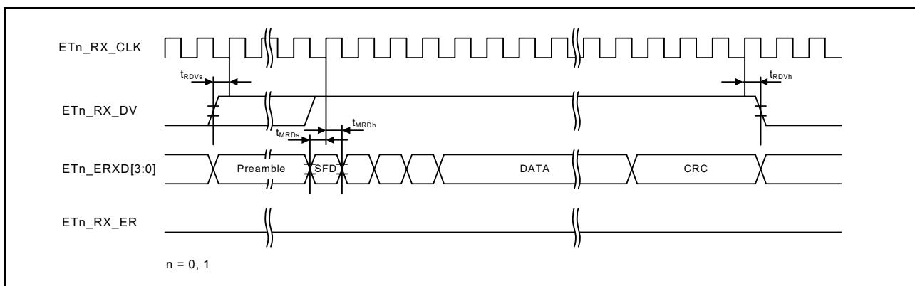
Figure 2.67 MII reception timing in normal operation
