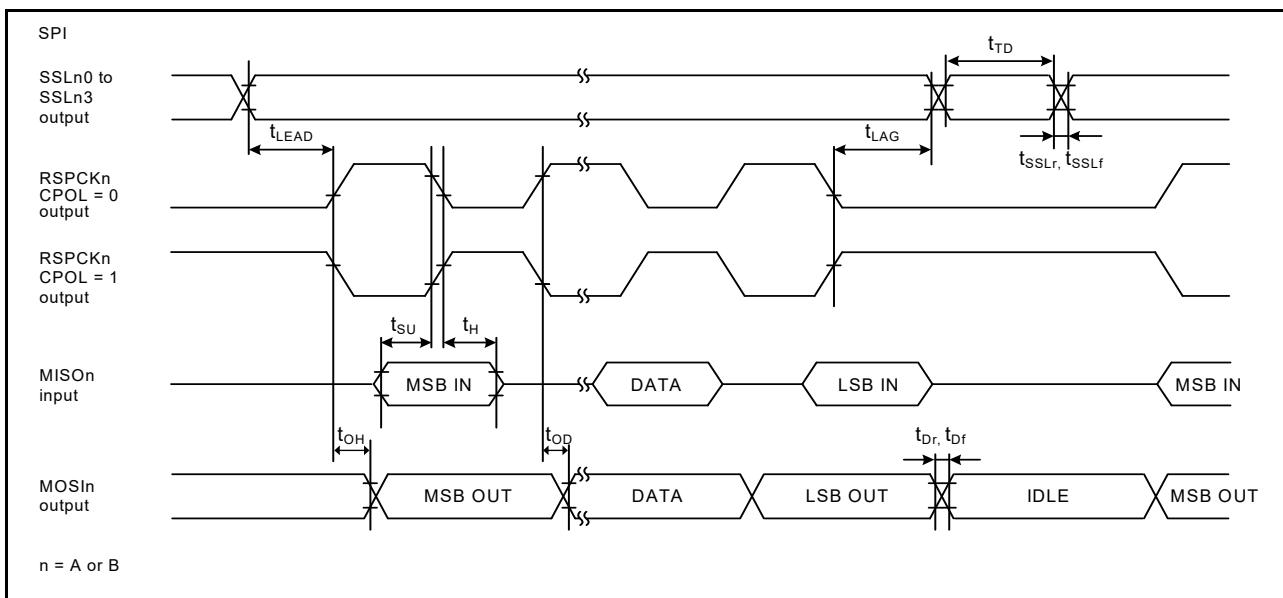
Figure 2.48 SPI timing for master when CPHA = 1
