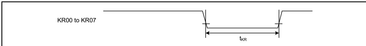
Figure 2.36 Key interrupt input timing
