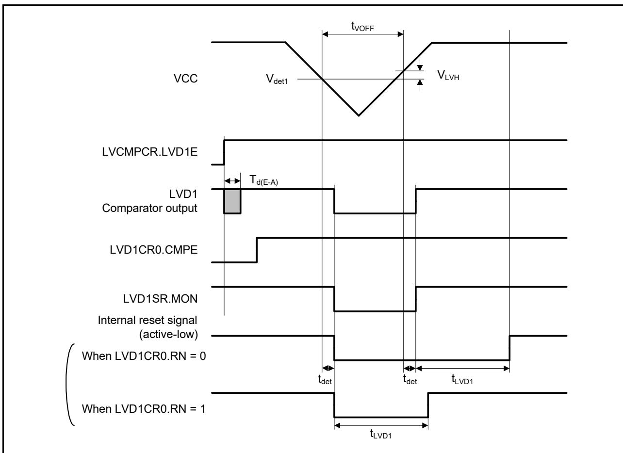
Figure 2.92 Voltage detection circuit timing ( $V_{det1}$ )
