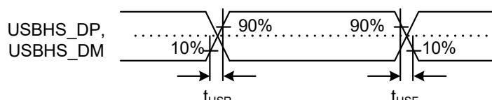
Figure 2.82 USBHS\_DP and USBHS\_DM output timing in high-speed mode
