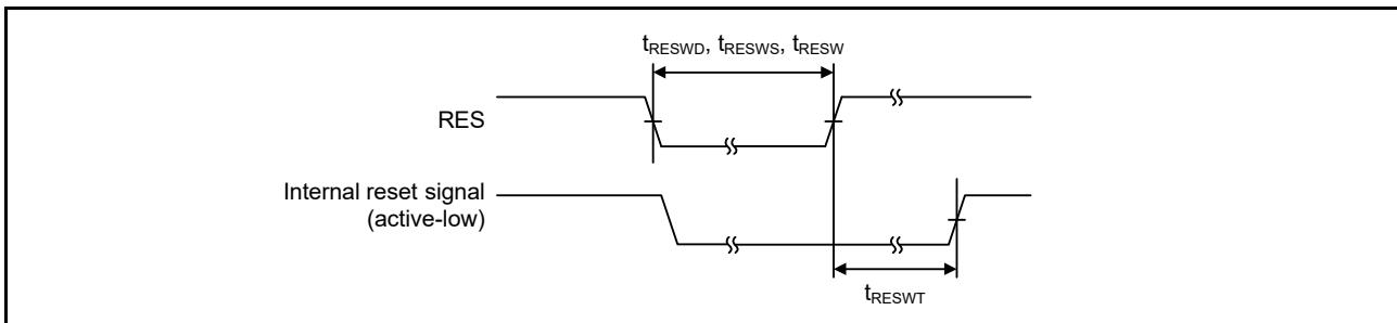
Figure 2.10 Reset input timing
