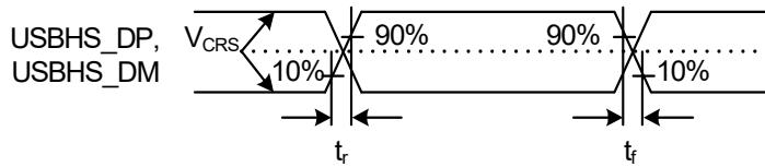
Figure 2.76 USBHS\_DP and USBHS\_DM output timing in low-speed mode
