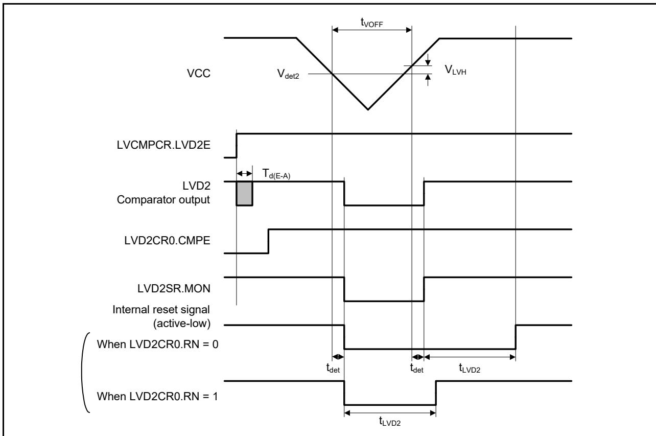
Figure 2.93 Voltage detection circuit timing ( $V_{det2}$ )
