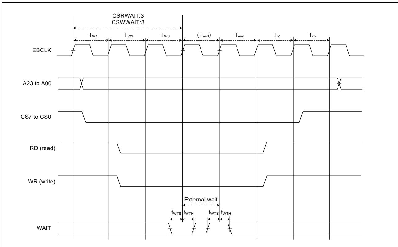
Figure 2.20 External bus timing for external wait control
