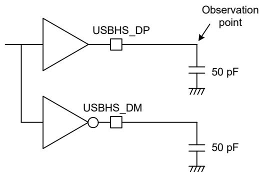
Figure 2.79 Test circuit in full-speed mode
