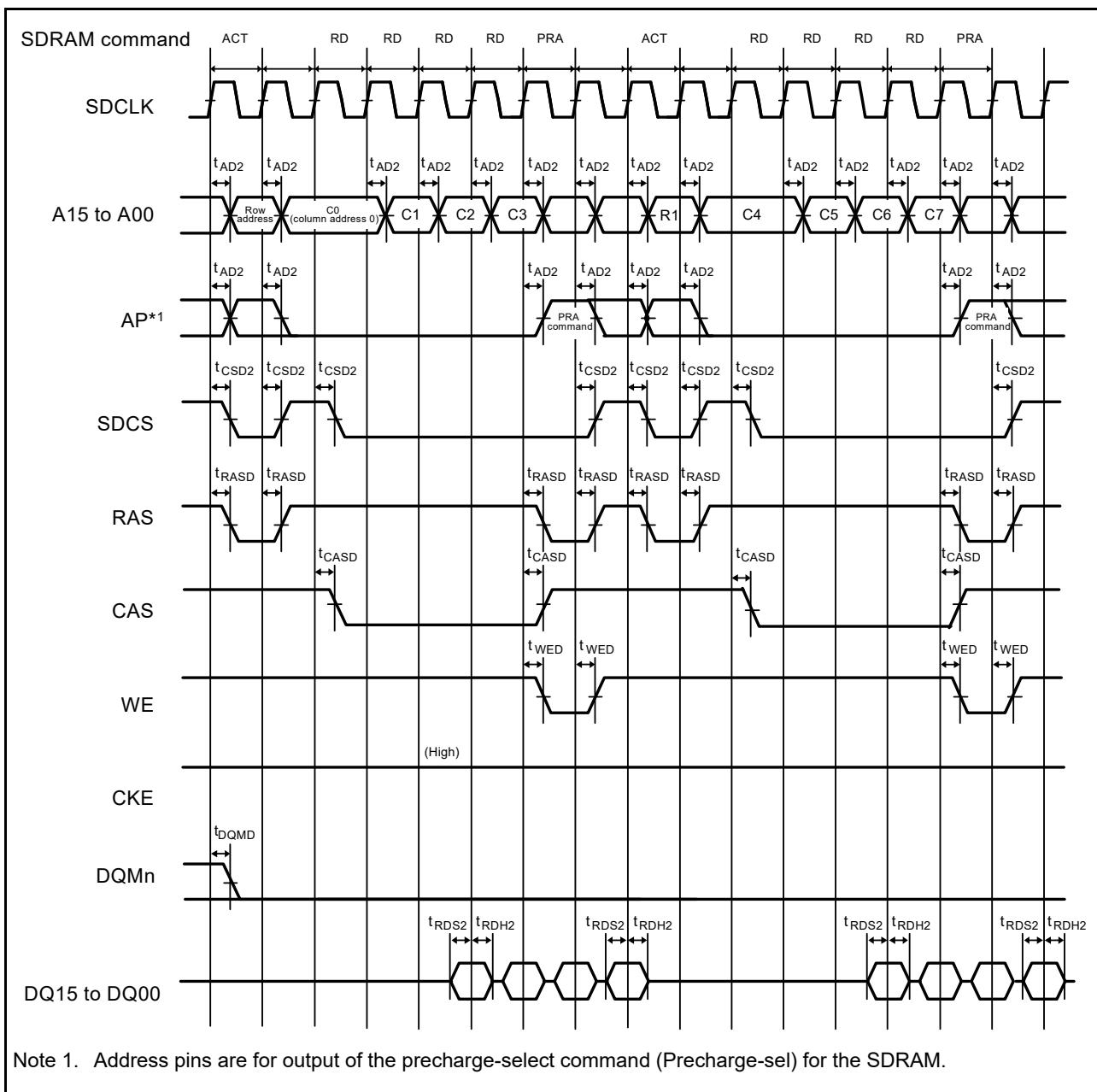
**Figure 2.25 SDRAM multiple read line stride timing**
