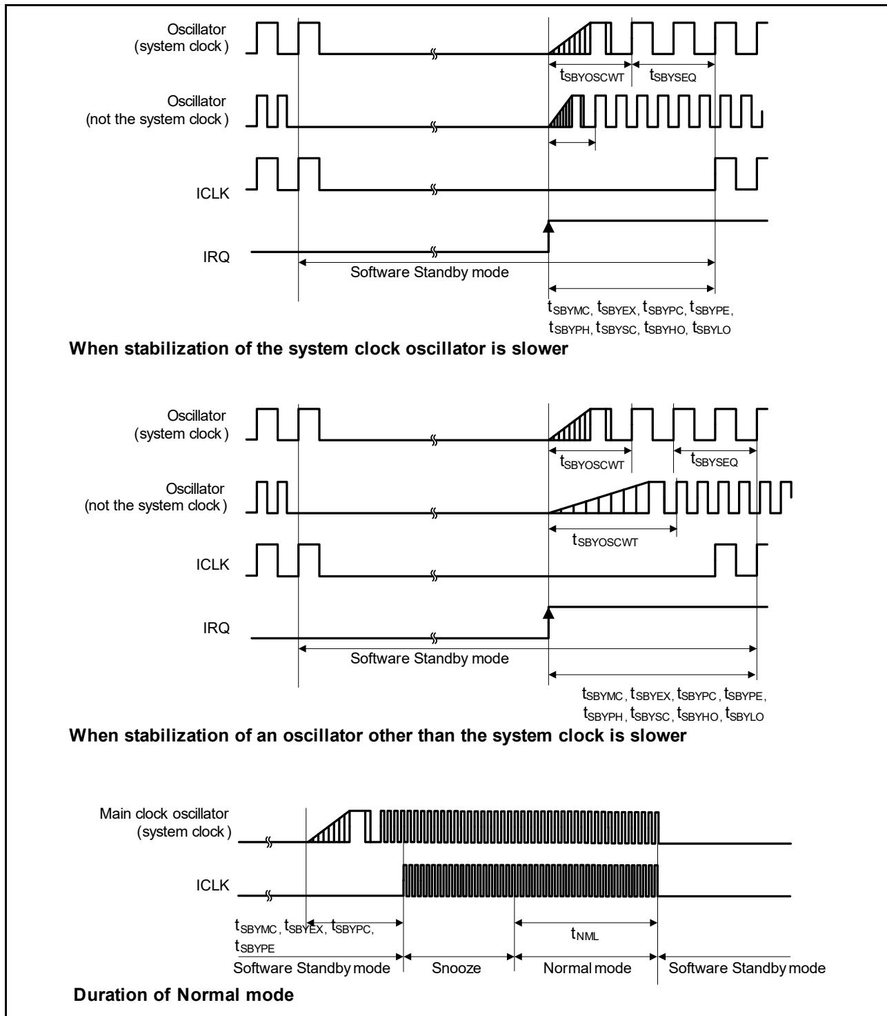
Figure 2.11 Software Standby mode cancellation timing and duration
