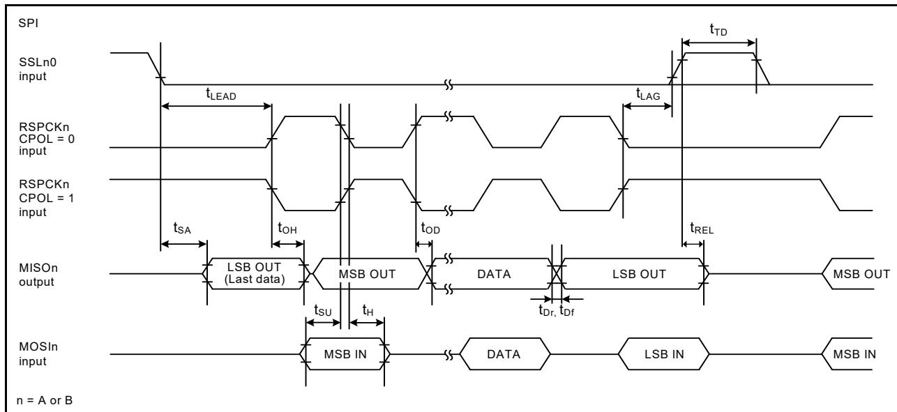
**Figure 2.51 SPI timing for slave when  $\text{CPHA} = 1$**
