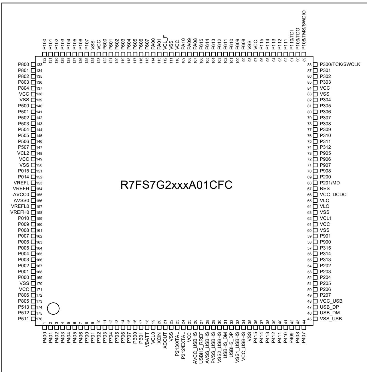
Figure 1.5 Pin assignment for 176-pin LQFP (top view)
