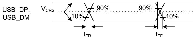
**Figure 2.86 USB\_DP and USB\_DM output timing in full-speed mode**
