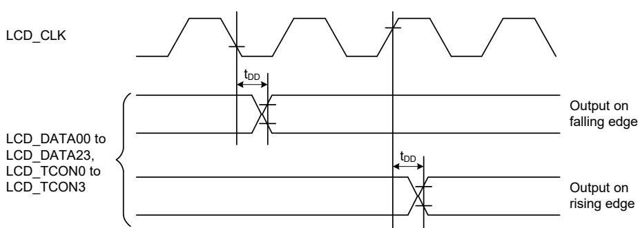
**Figure 2.75 Display output timing**
