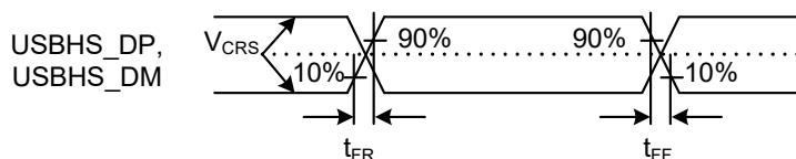
Figure 2.78 USBHS\_DP and USBHS\_DM output timing in full-speed mode
