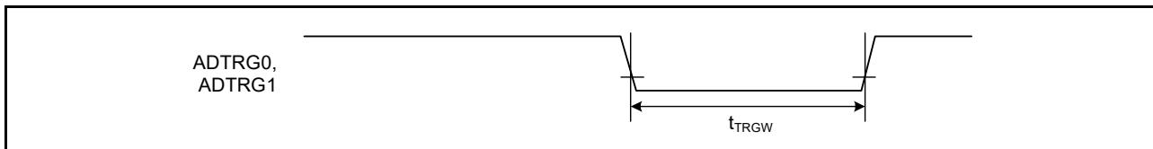
Figure 2.35 ADC12 trigger input timing
