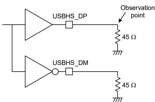
Figure 2.83 Test circuit in high-speed mode
