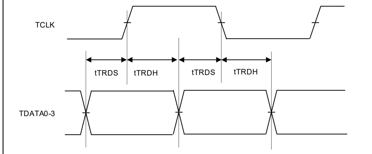
**Figure 2.104 ETM output timing**
