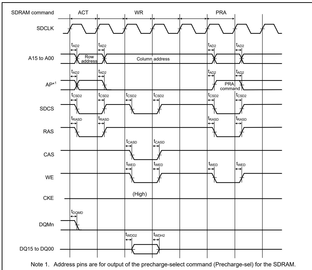
Figure 2.22 SDRAM single write timing
