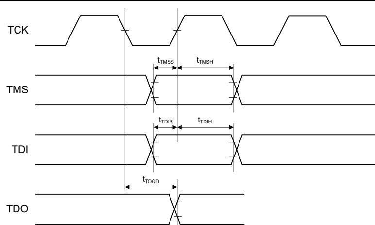
**Figure 2.97**    **Boundary scan input/output timing**
