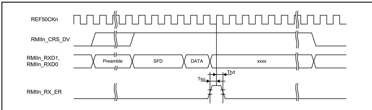
Figure 2.63 RMII reception timing when an error occurs
