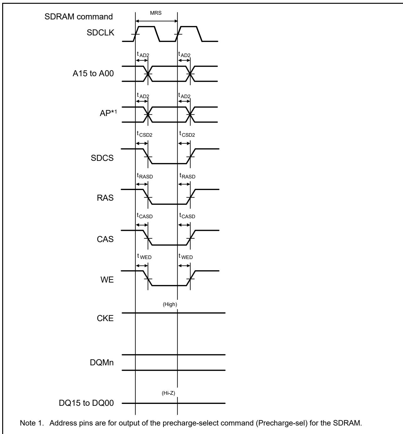
Figure 2.26 SDRAM mode register set timing
