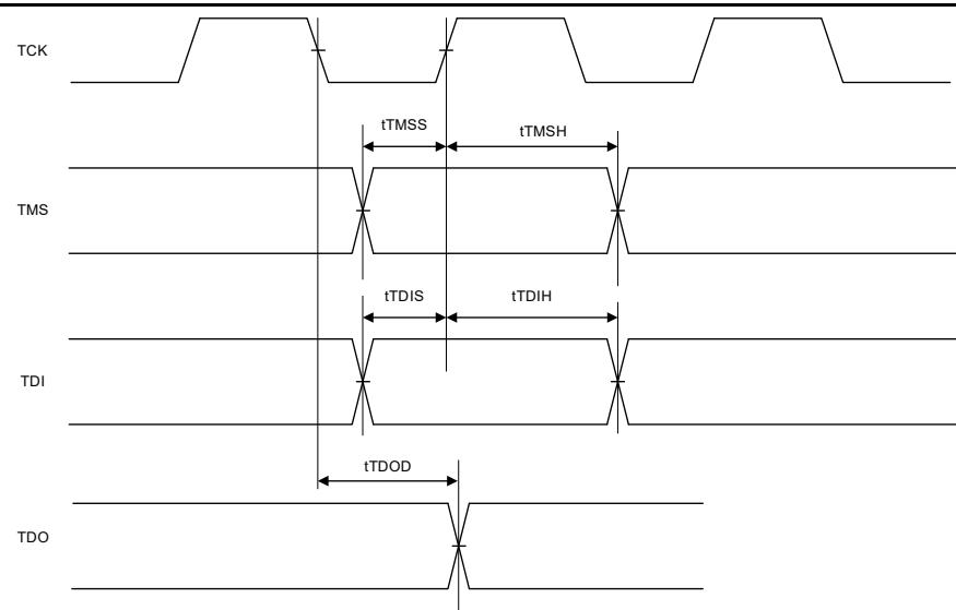
**Figure 2.100 JTAG input/output timing**
