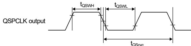
**Figure 2.52 QSPI clock timing**
