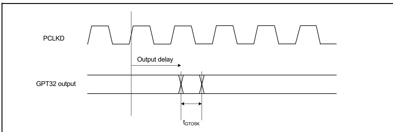
Figure 2.32 GPT32 output delay skew for OPS
