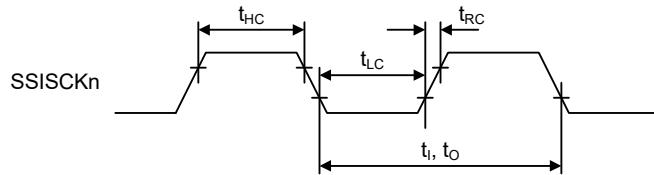
**Figure 2.55 SSI clock input/output timing**
