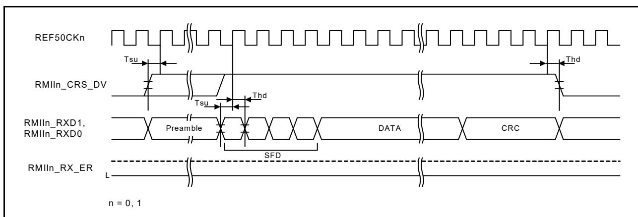
Figure 2.62 RMII reception timing in normal operation
