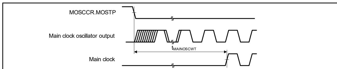
**Figure 2.5 Main clock oscillation start timing**
