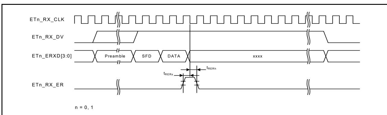
Figure 2.68 MII reception timing when an error occurs
