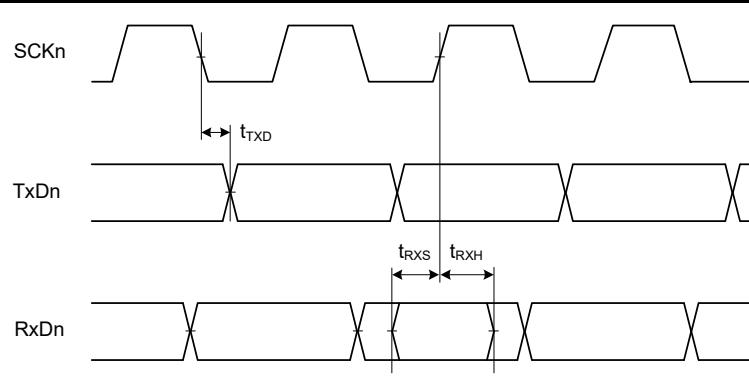
Figure 2.38 SCI input/output timing in clock synchronous mode
