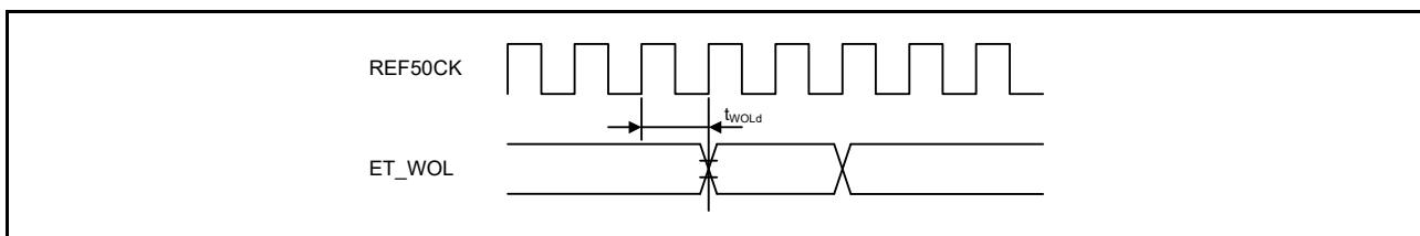
Figure 2.64 WOL output timing for RMII
