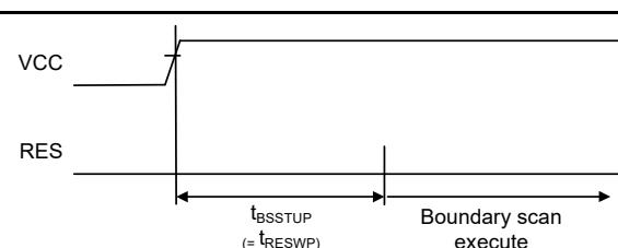
**Figure 2.98**    **Boundary scan circuit startup timing**
