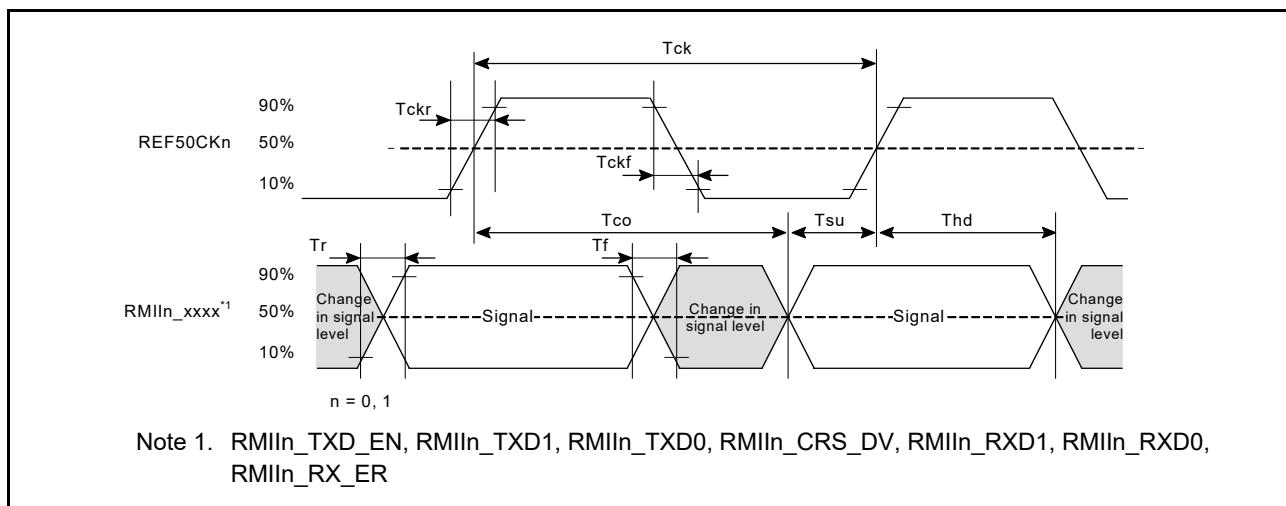
Figure 2.60 REF50CKn and RMII signal timing ( $n = 0$  and  $1$ )
