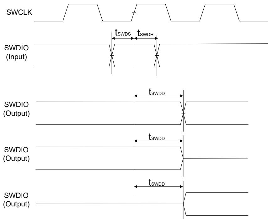
**Figure 2.102 SWD input/output timing**
