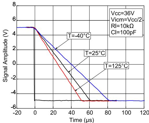
Figure 20: Positive slew rate behavior vs. temperature at VCC = 36 V
