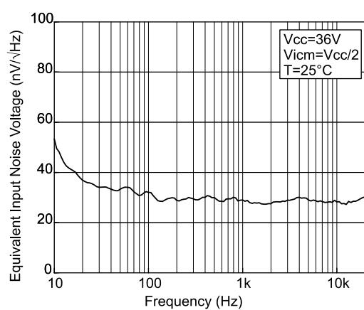
Figure 29: Noise vs. time at VCC = 36 V
