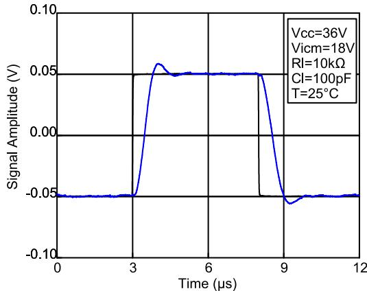
Figure 22: Output desaturation vs. time
