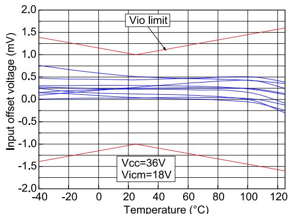
Figure 6: Input offset voltage temperature variation distribution at VCC = 36 V
