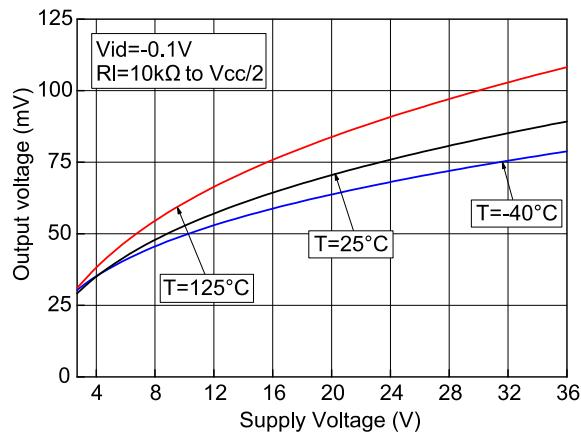
Figure 16: Amplifier behavior close to negative rail at VCC = 5 V
