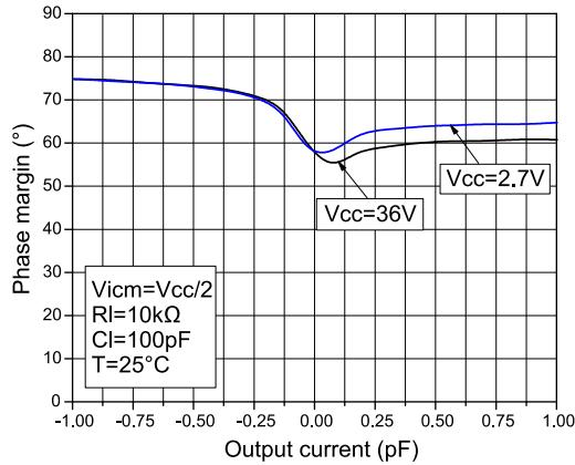
Figure 26: Phase margin vs. capacitive load at VCC = 2.7 V and 36 V
