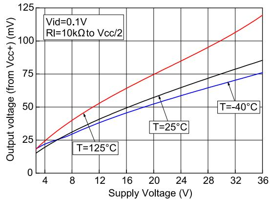
Figure 15: Output voltage (Vol) vs. supply voltage
