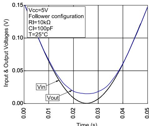
Figure 17: Amplifier behavior close to positive rail at VCC = 5 V
