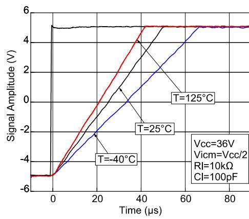
Figure 21: Small step response vs. time at VCC = 36 V
