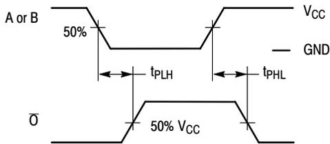
Figure 3. Switching Waveforms
