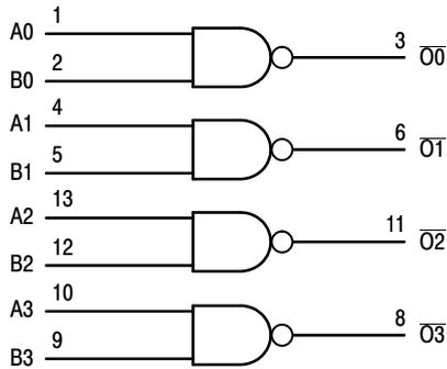
Figure 2. Logic Diagram
