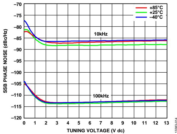
Figure 14. SSB Phase Noise vs. Tuning Voltage
