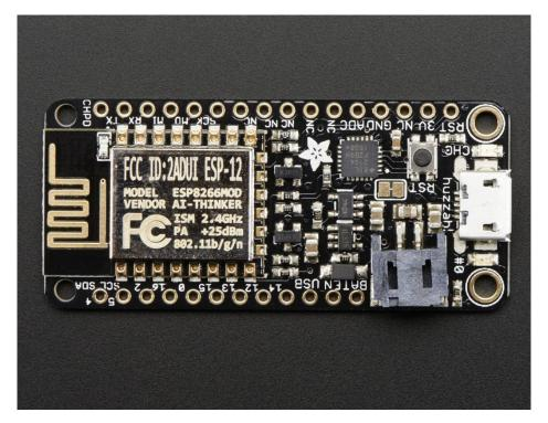
While the Feather HUZZAH ESP8266 comes pre-programmed with NodeMCU's Lua interpretter, you don't have to use it! Instead, you can use the Arduino IDE which may be more familar. This will write directly to the firmware, erasing the NodeMCU firmware, so if you want to go back to Lua, use the flasher to re-install it (https://adafru.it/f10)
