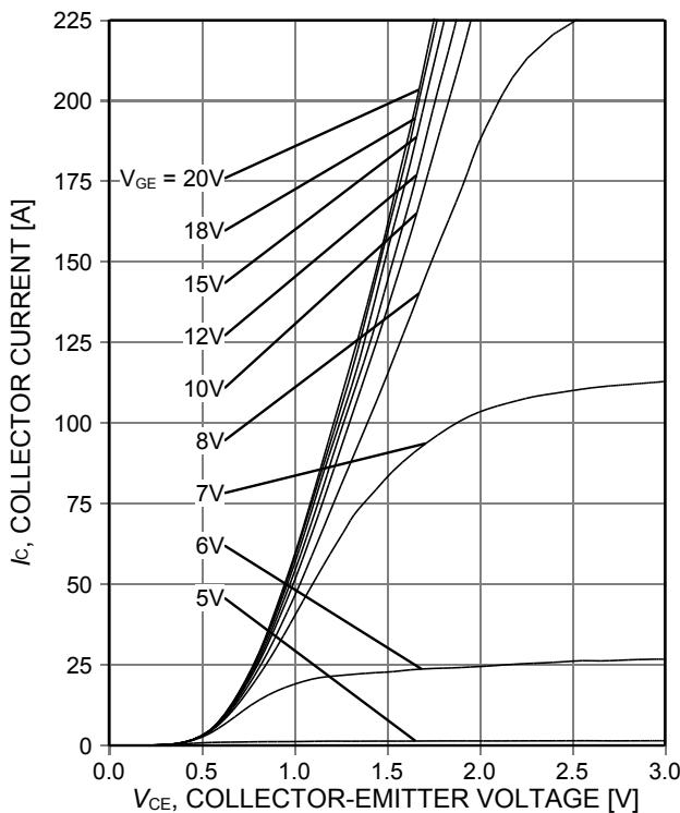
**Figure 5. Typical output characteristic**
