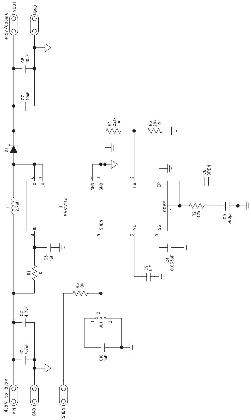
Figure 1. MAX17112 EV Kit Schematic
