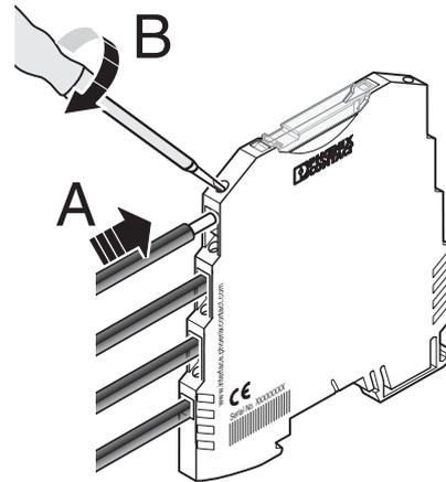
Figure 4 Screw connection
