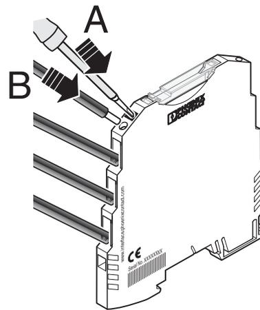
Figure 5 Spring-cage connection
