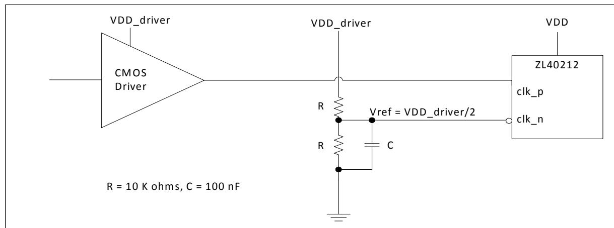
**Figure 10 - CMOS Input DC Coupled Referenced to VDD/2**
