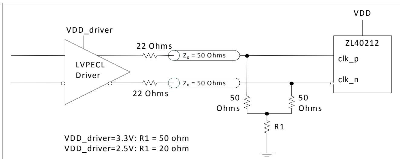
**Figure 4 - LVPECL Input DC Coupled Parallel Termination**
