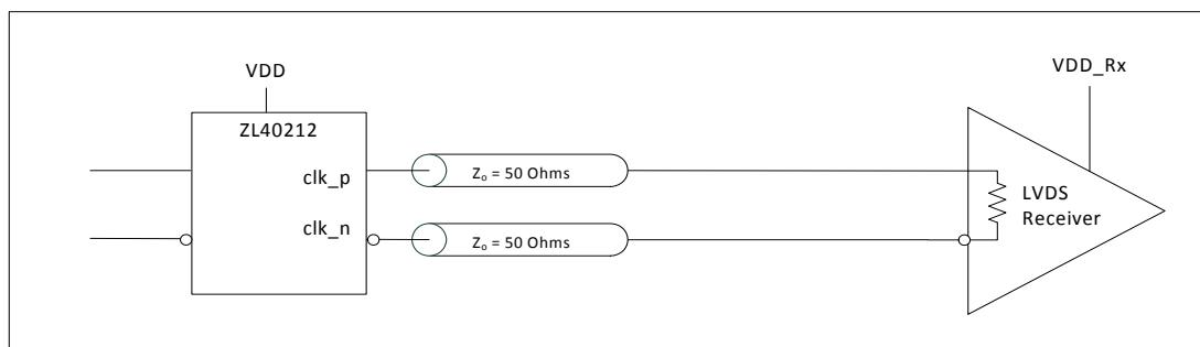
**Figure 13 - LVDS DC Coupled Termination (Internal Receiver Termination)**
