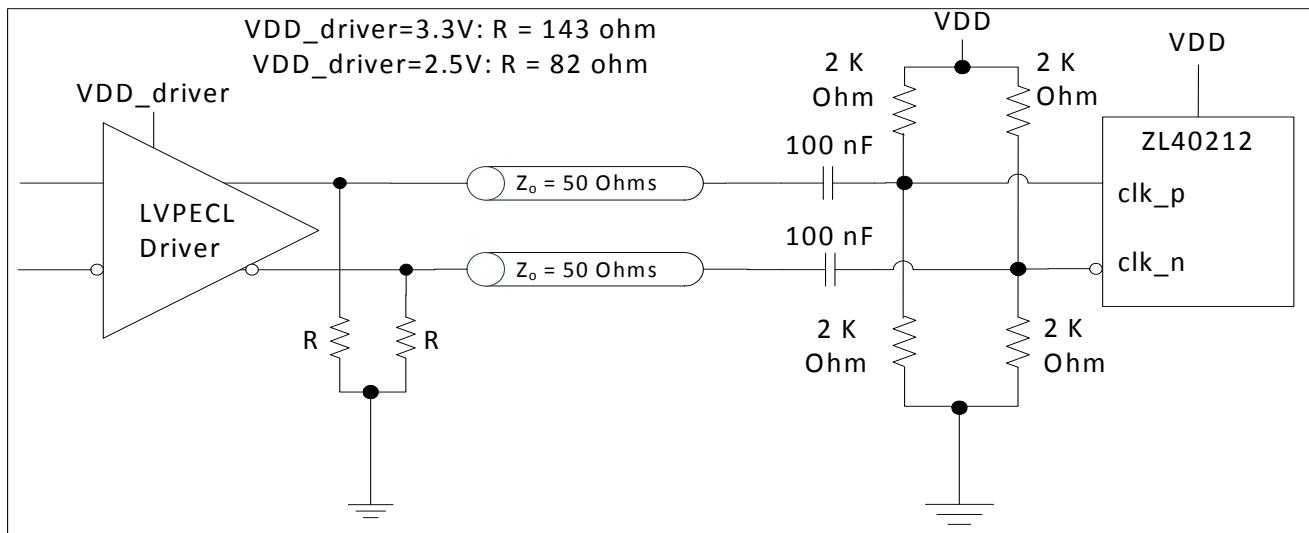
**Figure 5 - LVPECL Input AC Coupled Termination**
