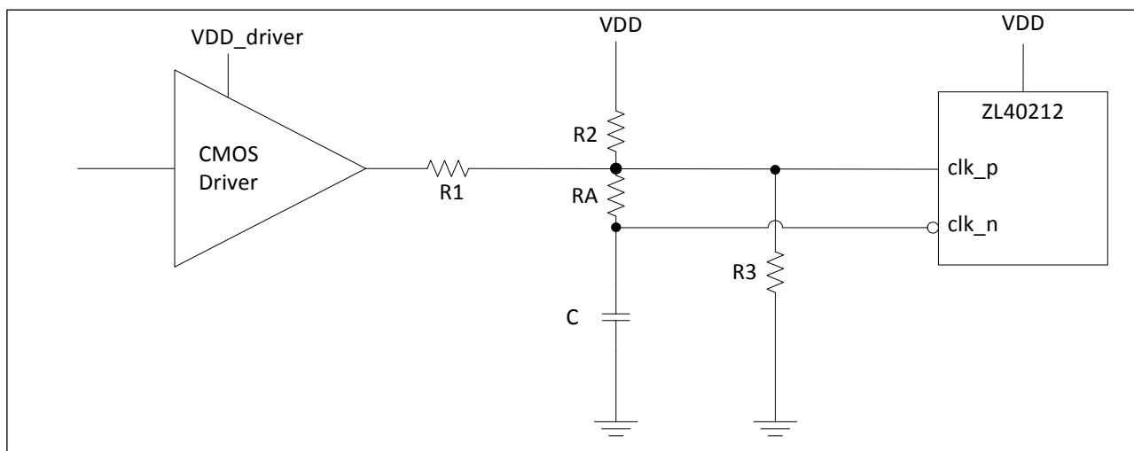
**Figure 11 - CMOS Input DC Coupled Referenced to Ground**
