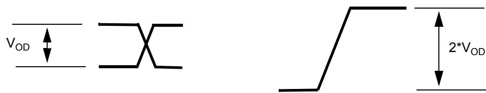
Figure 19 - Differential Output Voltage Parameter
