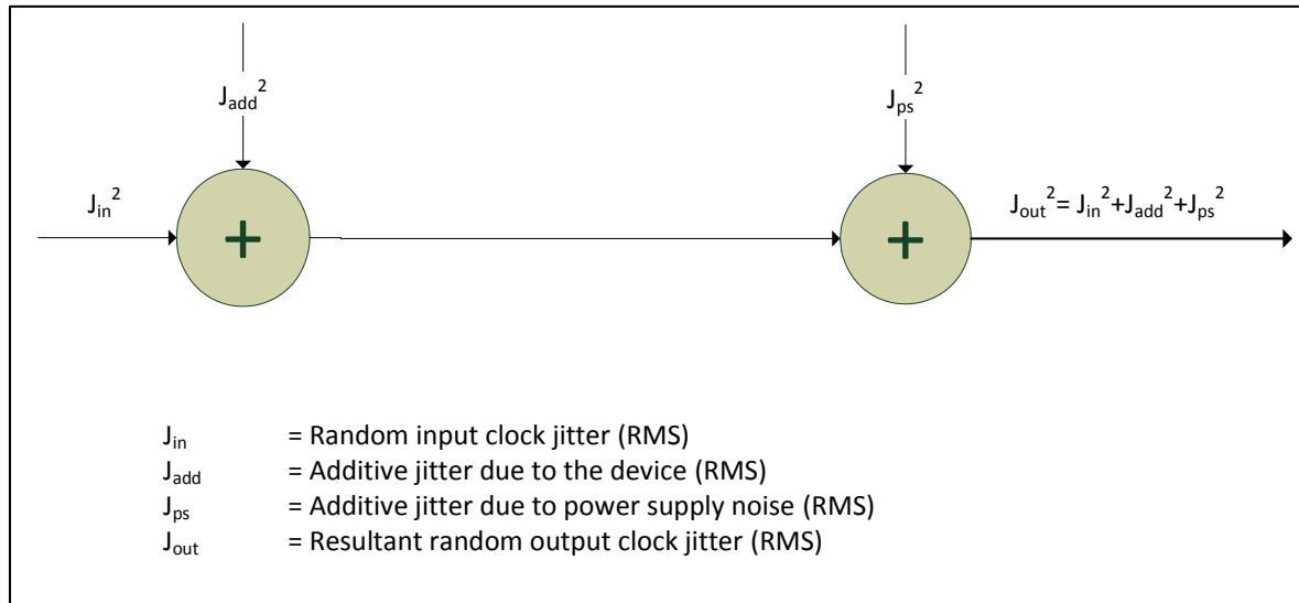
**Figure 17 - Additive Jitter**
