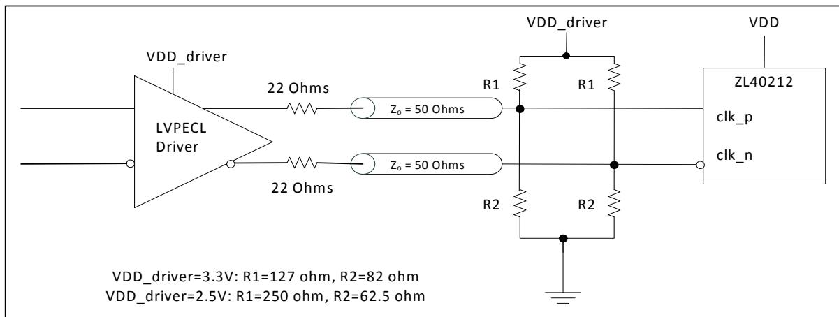
**Figure 3 - LVPECL Input DC Coupled Thevenin Equivalent**
