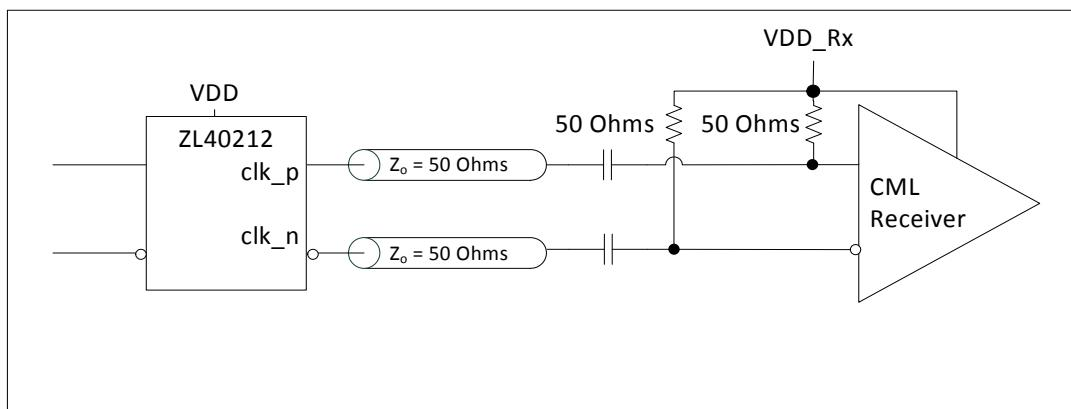
**Figure 16 - LVDS AC Output Termination for CML Inputs**
