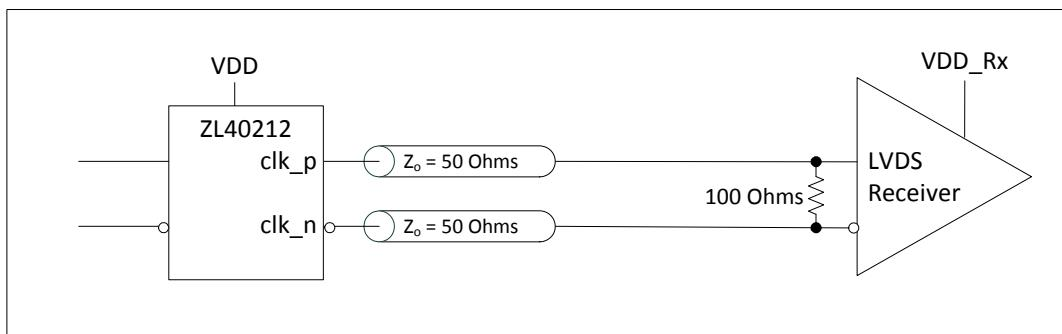
**Figure 14 - LVDS DC Coupled Termination (External Receiver Termination)**
