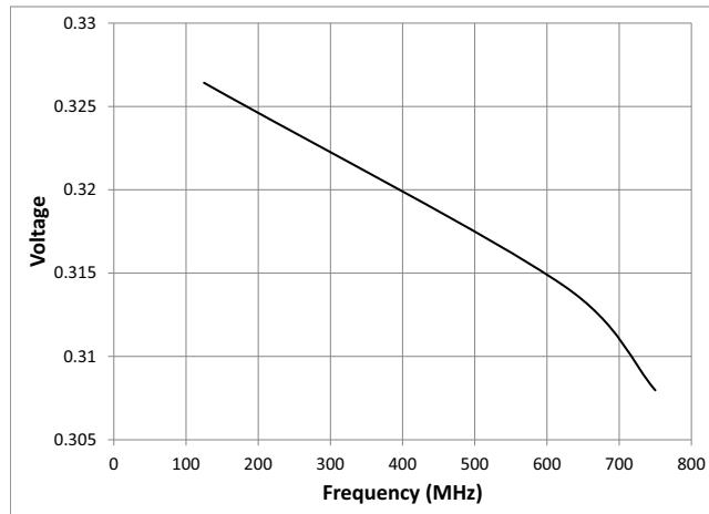
$V_{OD}$  versus Frequency
