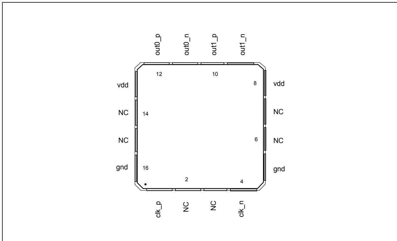
**Figure 2 - Pin Connections**
