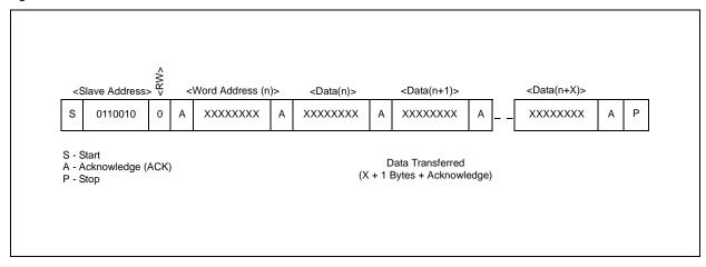
Figure 27. Data Read (Write Pointer, Then Read) - Slave Receive and Transmit
