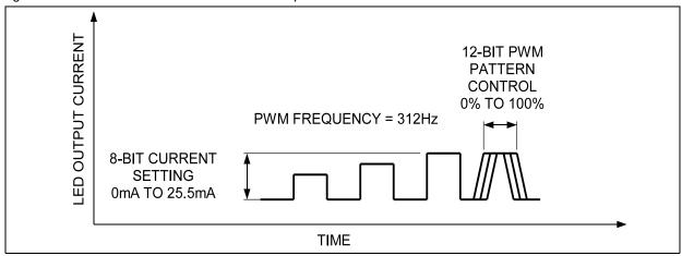
LED dimming is controlled according to a logarithmic or linear scale(see Figure 24). Logarithmic or linear scheme can be set for both the program execution engine control and direct PWM control.
