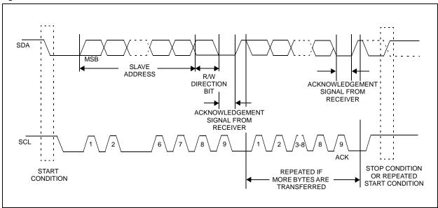
Figure 25. Data Transfer on PC Serial Bus
