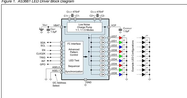
Figure 1. AS3661 LED Driver Block Diagram
