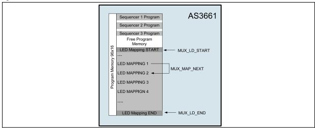
If the mapping table end address is reached, activation will roll to the mapping table start address next time when the mux\_map\_next instruction is called. Engine will not push a new PWM value to the LED driver output before set\_pwm or ramp instruction is executed. If the mapping has been released from an LED, the value in the PWM register will still control the LED brightness. If the mapping is released from the GPO pin, serial bus control takes over the GPO state.
