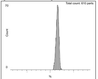
Figure 9. LED current Accuracy distribution @17.5mA
