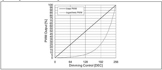
Note: If the temperature compensation is active, the maximum PWM duty cycle is limited to 50% at +25℃. This is required to allow enough headroom for temperature compensation over the whole temperature range -40 ℃ to 90℃.
