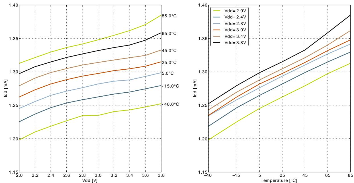
**Figure 3.7. EM1 Current consumption with all peripheral clocks disabled and HFRCO running at 21MHz**
