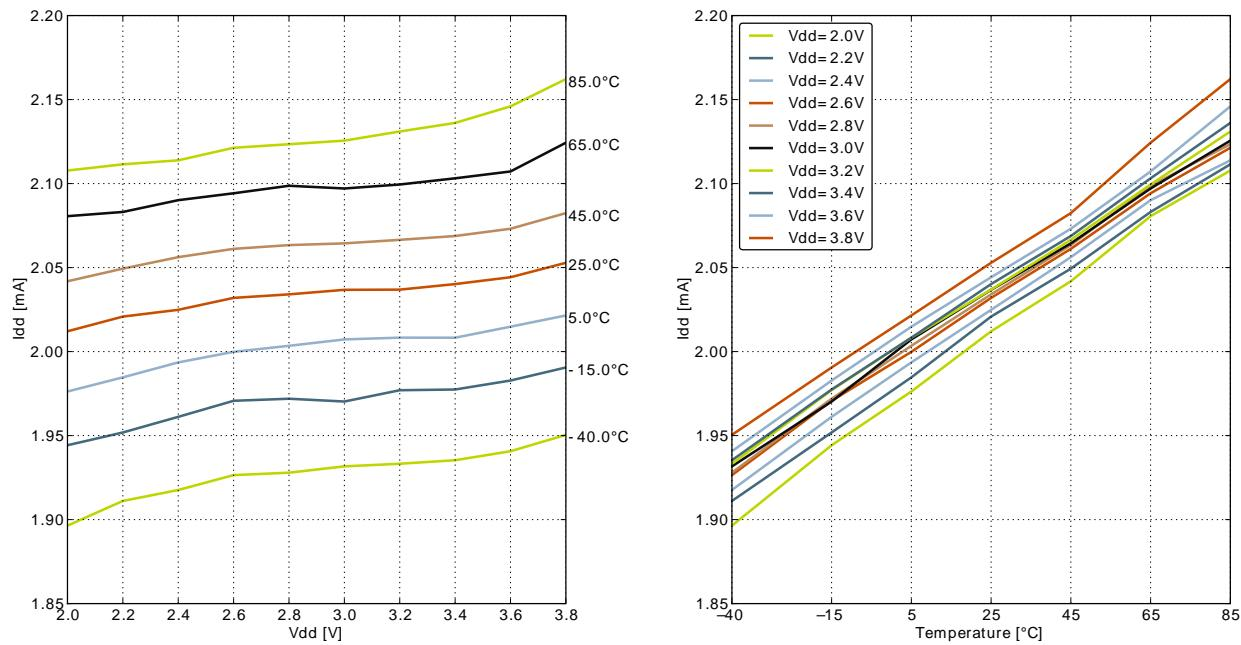
**Figure 3.5. EM0 Current consumption while executing prime number calculation code from flash with HFRCO running at 7MHz**
