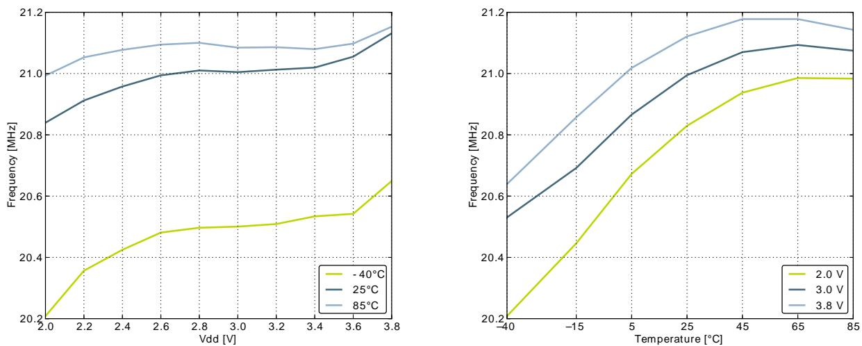
**Figure 3.26. Calibrated HFRCO 28 MHz Band Frequency vs Supply Voltage and Temperature**
