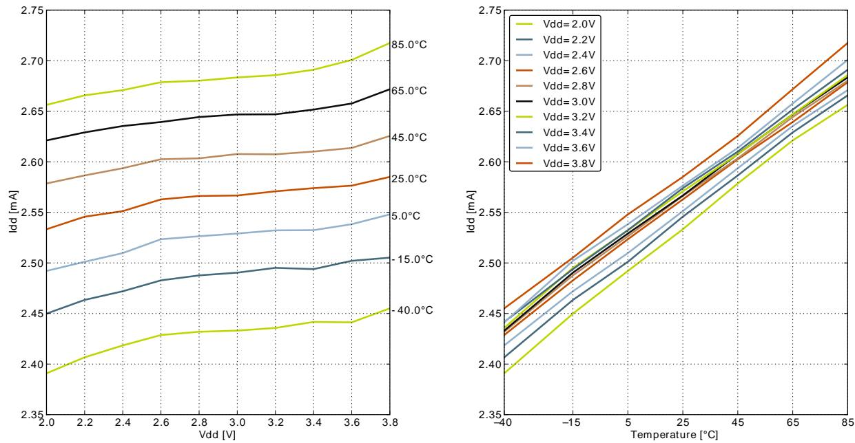
**Figure 3.4. EMO Current consumption while executing prime number calculation code from flash with HFRCO running at 11MHz**
