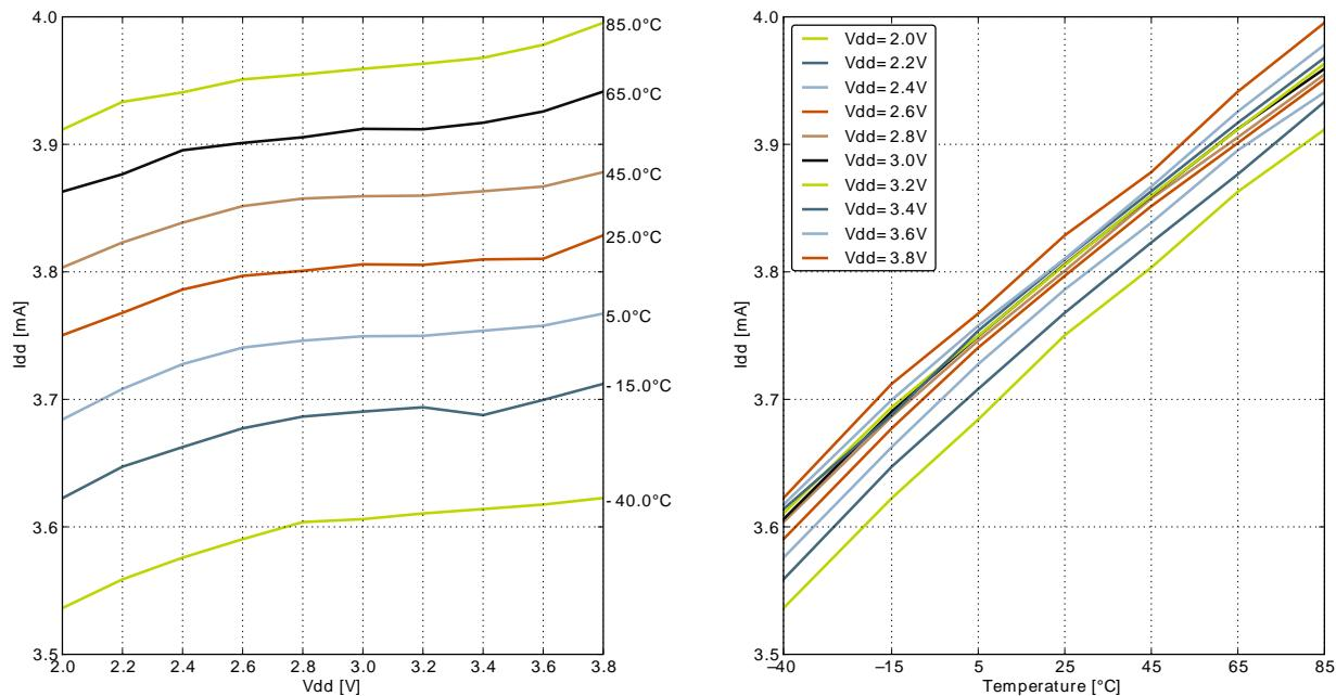
**Figure 3.3. EMO Current consumption while executing prime number calculation code from flash with HFRCO running at 14MHz**
