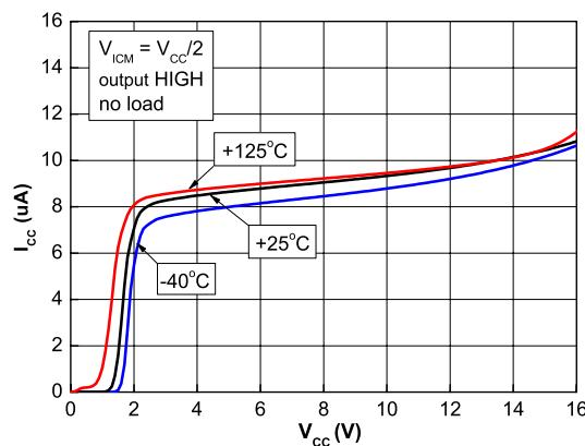
**Figure 4. Current consumption vs. supply voltage, output low**
