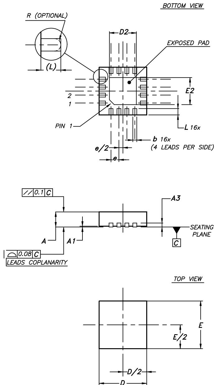
Note: The exposed pad is not internally connected and can be set to ground or left floating.
