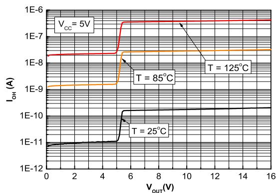
**Figure 8. Output leakage current vs. supply voltage,  $V_{cc} = 5\text{ V}$**
