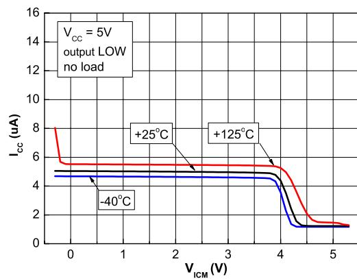
**Figure 7. Output leakage current vs. output voltage,  $V_{cc} = 5\text{ V}$**
