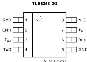
**Figure 1** Pin Configuration (top view)
