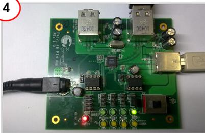
Connect a USB device to any of the four downstream ports. Use jumpers J7 to J10 (port status) in position 2 or 3 to enable the port LEDs. The green LED indicates that the port is enabled.
