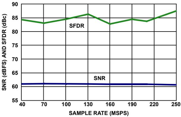
FIGURE 9. SNR AND SFDR vs f<sub>SAMPLE</sub>
