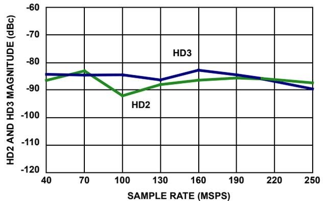
FIGURE 10. HD2 AND HD3 vs f<sub>SAMPLE</sub>
