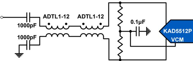
FIGURE 29. TRANSMISSION-LINE TRANSFORMER INPUT FOR HIGH IF APPLICATIONS
