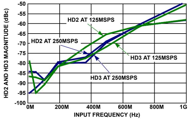
FIGURE 6. HD2 AND HD3 vs f<sub>IN</sub>
