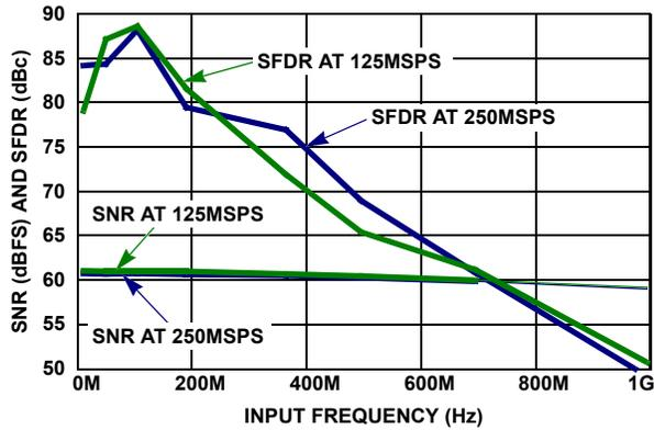
FIGURE 5. SNR AND SFDR vs f<sub>IN</sub>
