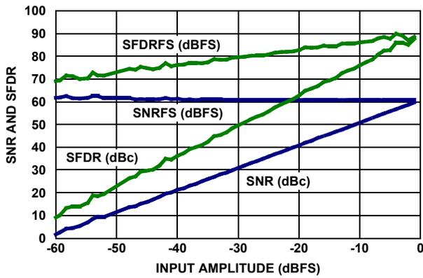
FIGURE 7. SNR AND SFDR vs A<sub>IN</sub>
