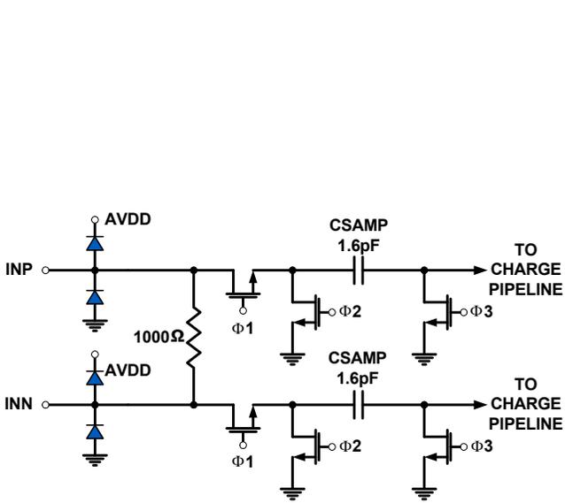
FIGURE 43. ANALOG INPUTS
