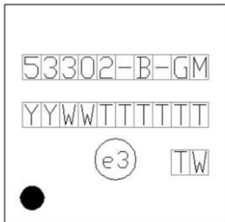
Figure 8.4. Si53302 Top Marking
