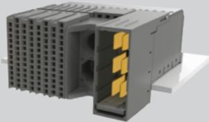
Power and keying/guidance modules also are available but require a single customizable BSP product. A BSP product is built by combining any number, in any configuration, of HDTFs, power and keying/guidance modules to create one receptacle. Contact HSBP@samtec.com for more information about building a BSP product.
