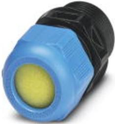
Cable gland, Cable gland material: Polyamide, Application: Ex, External cable diameter 13 mm ... 21 mm, Shielding: No, Connecting thread: M32, Color: black/blue
