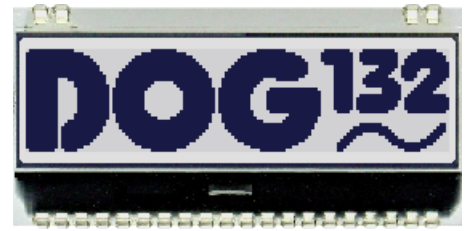
Orientation for 12 o'clock (Top View)
