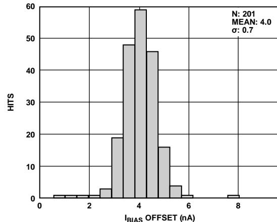
Figure 8. Typical Distribution of Input Offset Current
