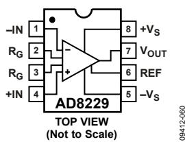
Figure 58. Pinout Diagram
