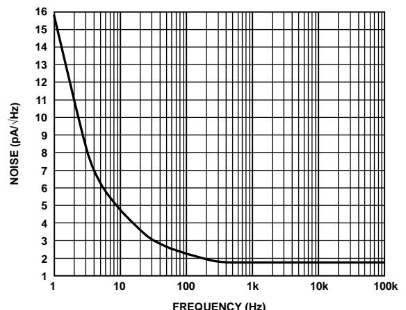
Figure 40. Current Noise Spectral Density vs. Frequency
