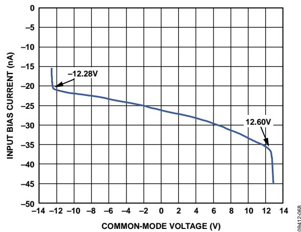
Figure 17. Input Bias Current vs. Common-Mode Voltage
