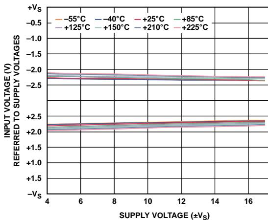
Figure 31. Input Voltage Limit vs. Supply Voltage
