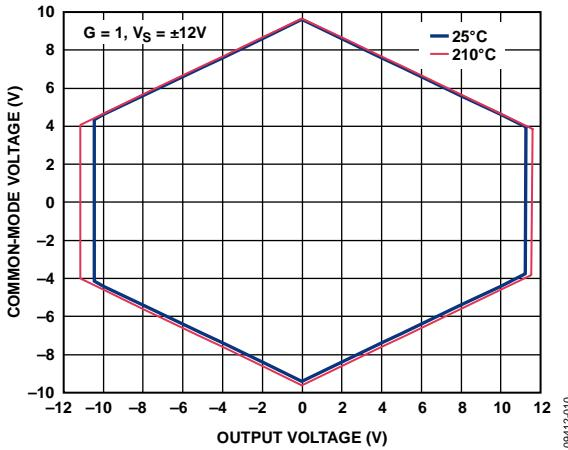
Figure 12. Input Common-Mode Voltage vs. Output Voltage,
