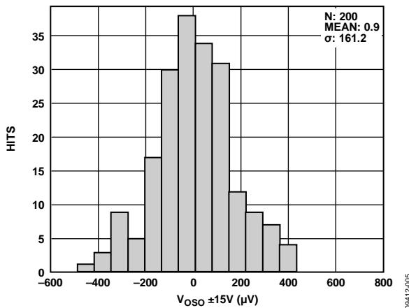
Figure 6. Typical Distribution of Output Offset Voltage
