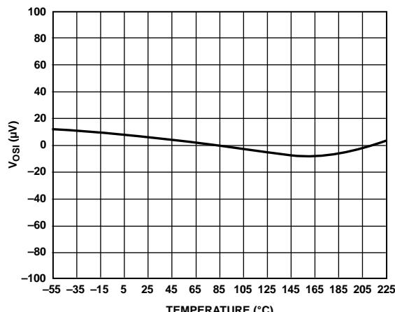
Figure 2. Typical Input Offset vs. Temperature (G = 100)
