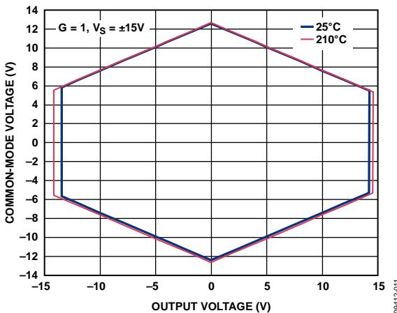
Figure 13. Input Common-Mode Voltage vs. Output Voltage,
