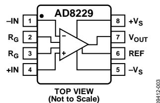
Figure 4. Pin Configuration
