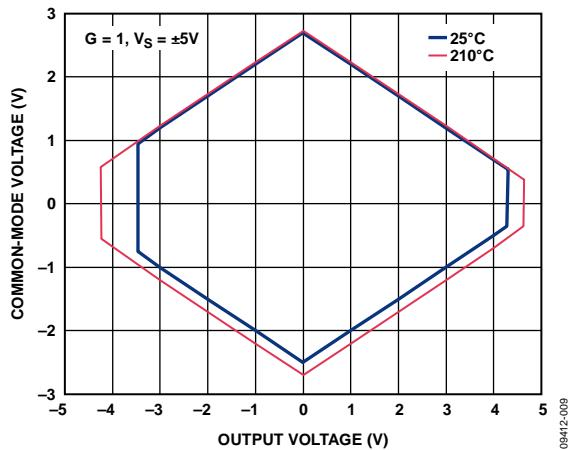
Figure 11. Input Common-Mode Voltage vs. Output Voltage,
