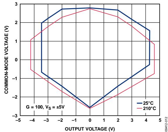
Figure 14. Input Common-Mode Voltage vs. Output Voltage,
