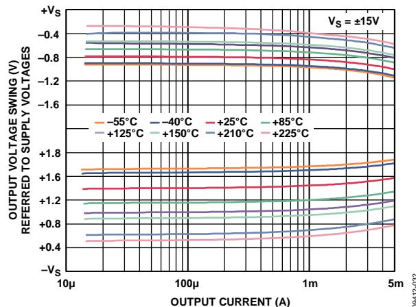
Figure 35. Output Voltage Swing vs. Output Current
