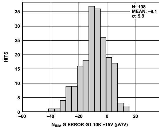
Figure 10. Typical Distribution of Gain Error,  $G = 1$
