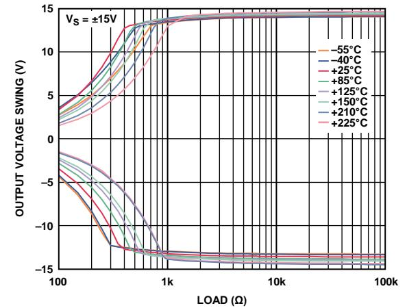
Figure 34. Output Voltage Swing vs. Load Resistance
