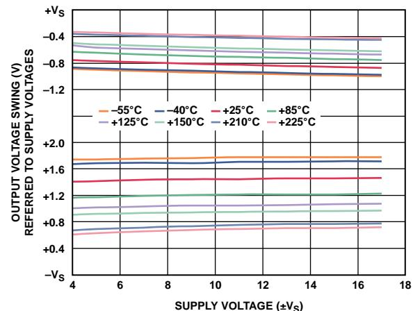
Figure 32. Output Voltage Swing vs. Supply Voltage,  $R_L = 10 k\Omega$
