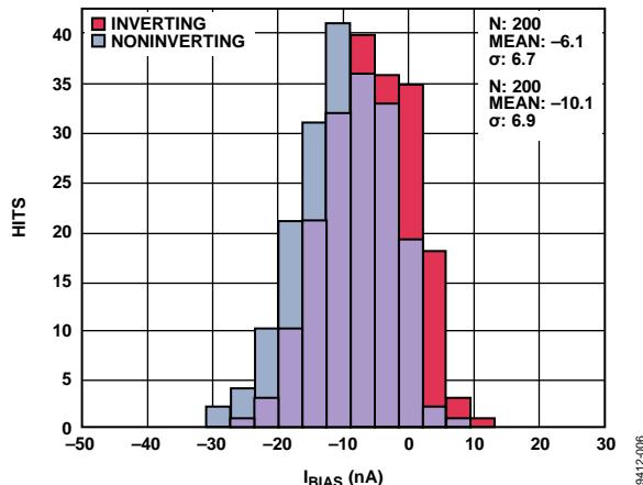
Figure 7. Typical Distribution of Input Bias Current
