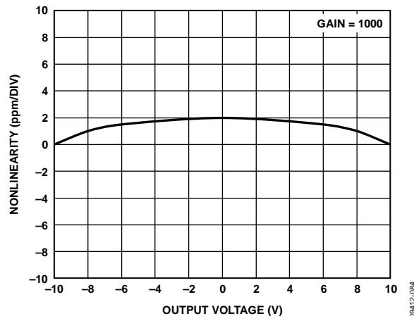
Figure 37. Gain Nonlinearity,  $G = 1000, R_L = 10\text{ k}\Omega$
