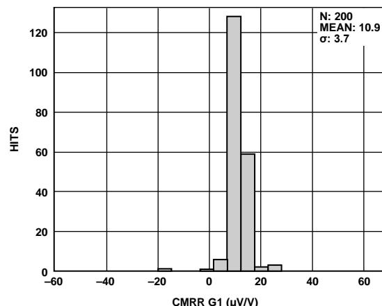
Figure 9. Typical Distribution of Common Mode Rejection,  $G = 1$
