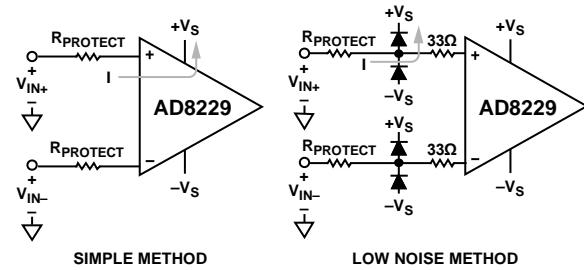
Figure 61. Protection for Voltages Beyond the Rails
