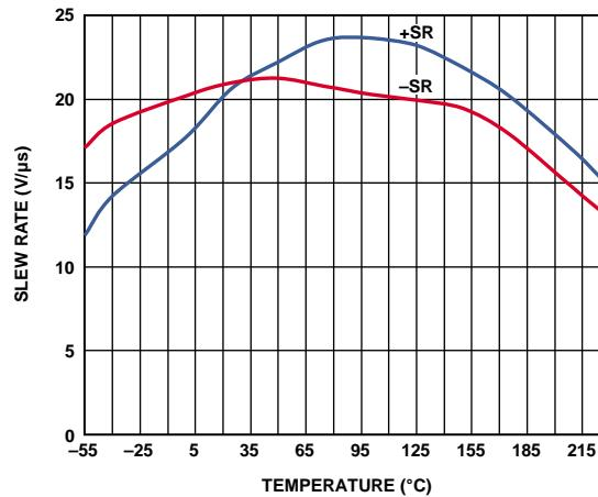
Figure 30. Slew Rate vs. Temperature,  $V_S = \pm 5 V, G = 1$
