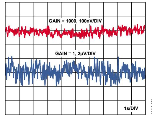
Figure 39. 0.1 Hz to 10 Hz RTI Voltage Noise,  $G = 1, G = 1000$
