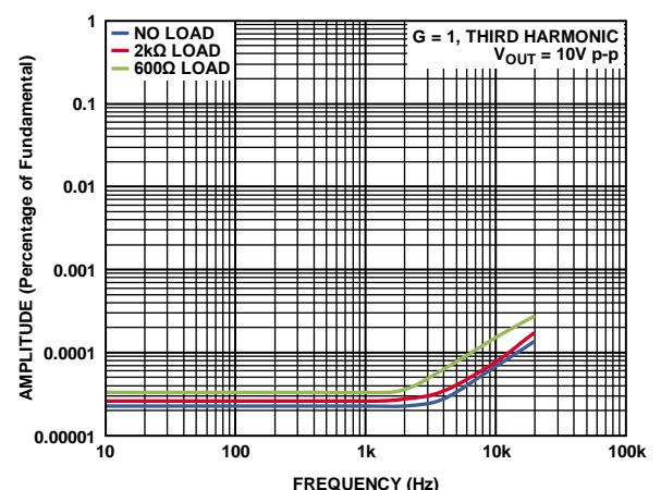
Figure 52. Third Harmonic Distortion vs. Frequency,  $G = 1$
