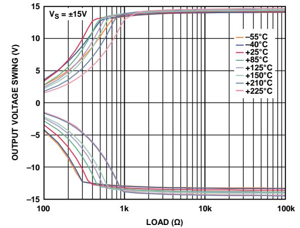
Figure 34. Output Voltage Swing vs. Load Resistance
