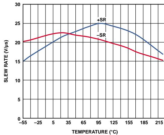
Figure 29. Slew Rate vs. Temperature,  $V_S = \pm 15 V, G = 1$
