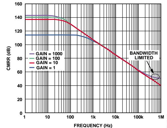
Figure 22. CMRR vs. Frequency, 1 kΩ Source Imbalance
