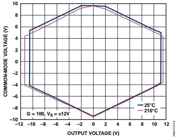
Figure 15. Input Common-Mode Voltage vs. Output Voltage,
