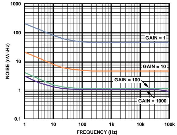
Figure 38. Voltage Noise Spectral Density vs. Frequency
