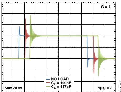
Figure 49. Small Signal Response with Various Capacitive Loads,  $G = 1$ ,  $R_L = \text{Infinity}$
