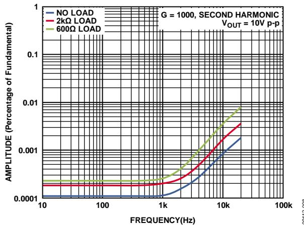
Figure 53. Second Harmonic Distortion vs. Frequency,  $G = 1000$
