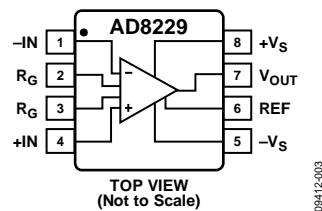
Figure 4. Pin Configuration
