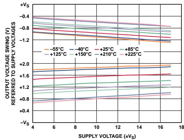
Figure 33. Output Voltage Swing vs. Supply Voltage,  $R_L = 2 k\Omega$
