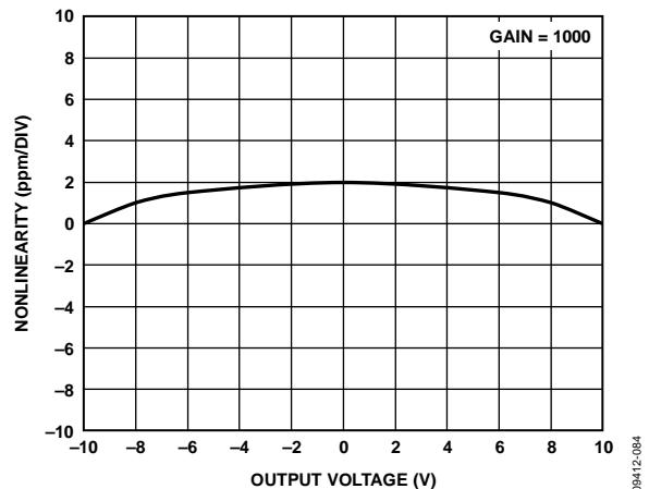
Figure 37. Gain Nonlinearity,  $G = 1000, R_L = 10\text{ k}\Omega$
