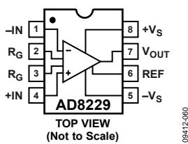
Figure 58. Pinout Diagram
