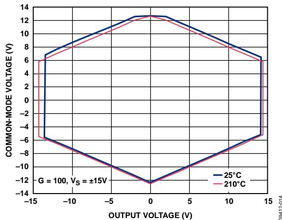
Figure 16. Input Common-Mode Voltage vs. Output Voltage,
