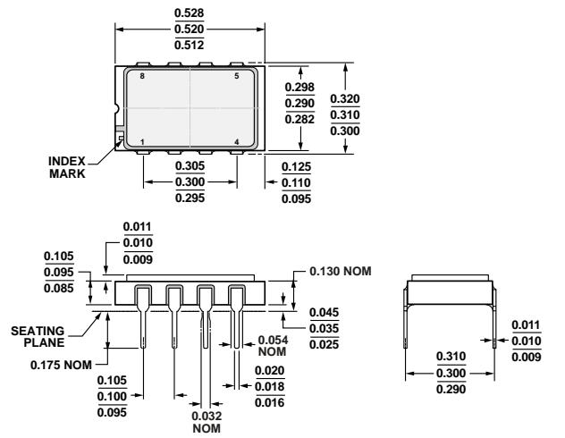
Figure 65. 8-Lead Side-Brazed Ceramic Dual In-Line Package [SBDIP]
