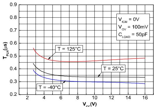
Figure 16: Propagation delay tPHL vs. supply voltage
