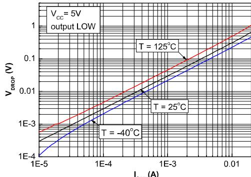
Figure 10: Output voltage drop vs. output sink current,
