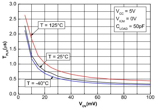
Figure 14: Propagation delay tPHL vs. input signal overdrive, V<sub>CC</sub> = 5 V
