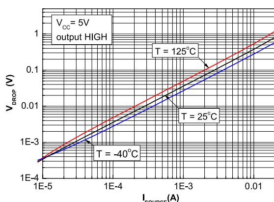
Figure 9: Output voltage drop vs. output sink current,
