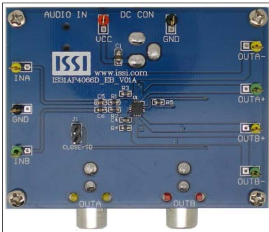
Figure 1: Photo of IS31AP4066D Evaluation Board
