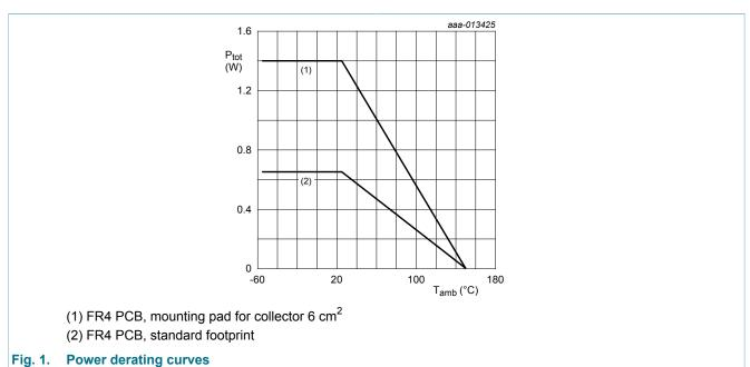
600 V, 0.5 A NPN high-voltage low VCEsat (BISS) transistor
