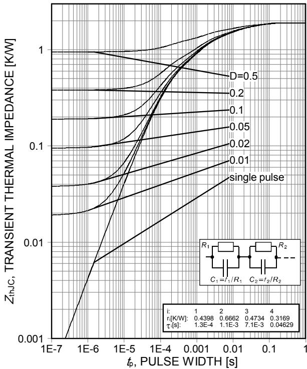
Figure 22. Diode transient thermal impedance as a function of pulse width
