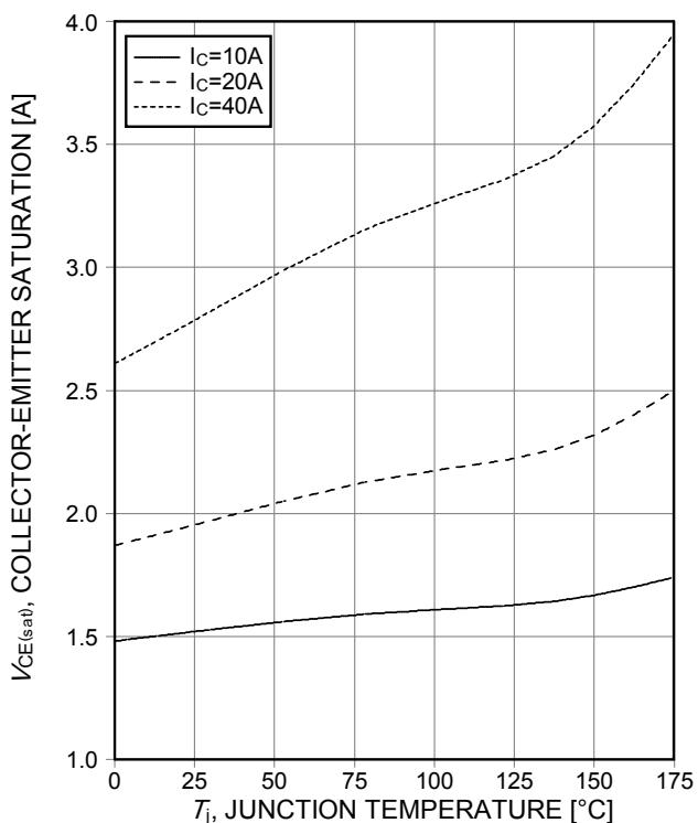
**Figure 8. Typical collector-emitter saturation voltage**
