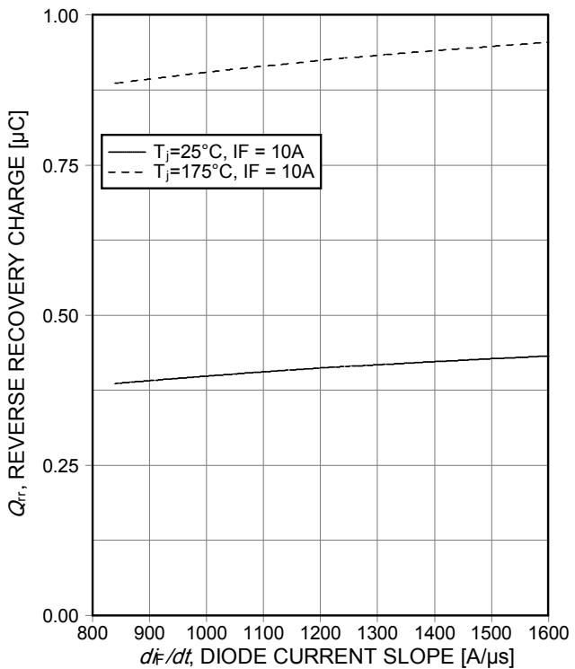
Figure 24. Typical reverse recovery charge as a function of diode current slope
