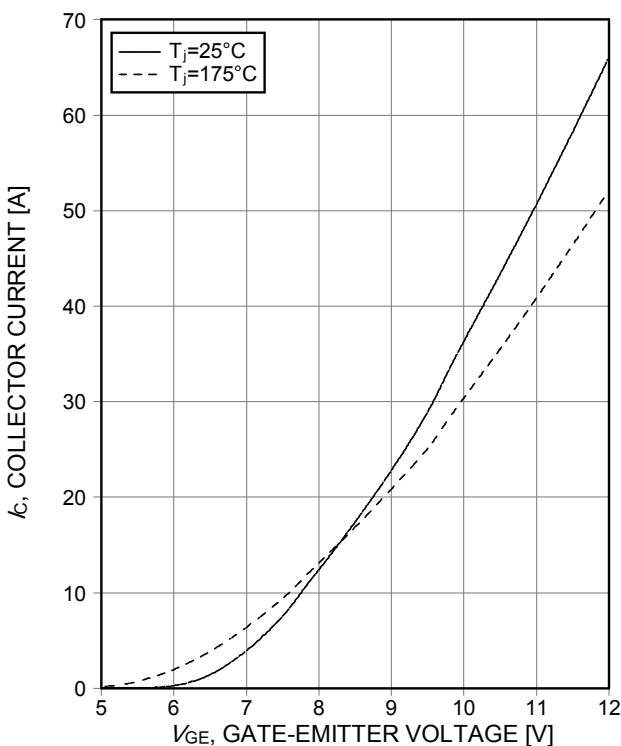
**Figure 7. Typical transfer characteristic**
