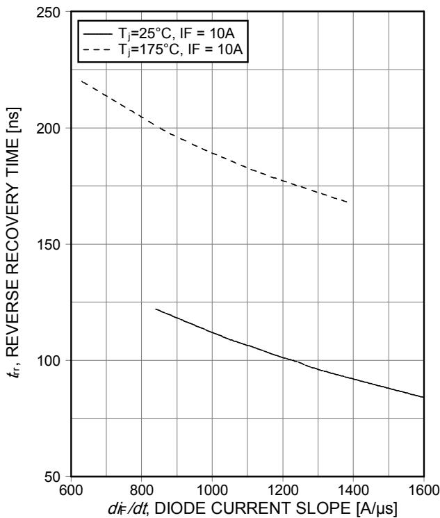
Figure 23. Typical reverse recovery time as a function of diode current slope
