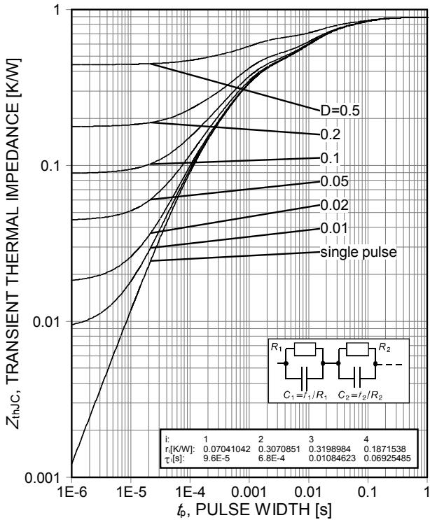
Figure 21. IGBT transient thermal impedance
