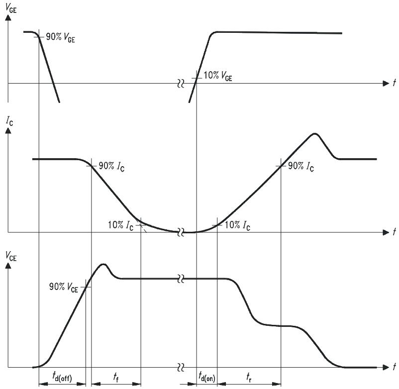
**Figure A. Definition of switching times**
