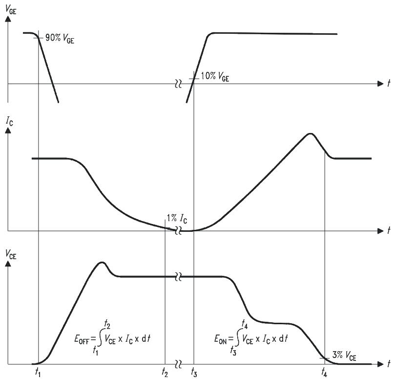
**Figure B. Definition of switching losses**
