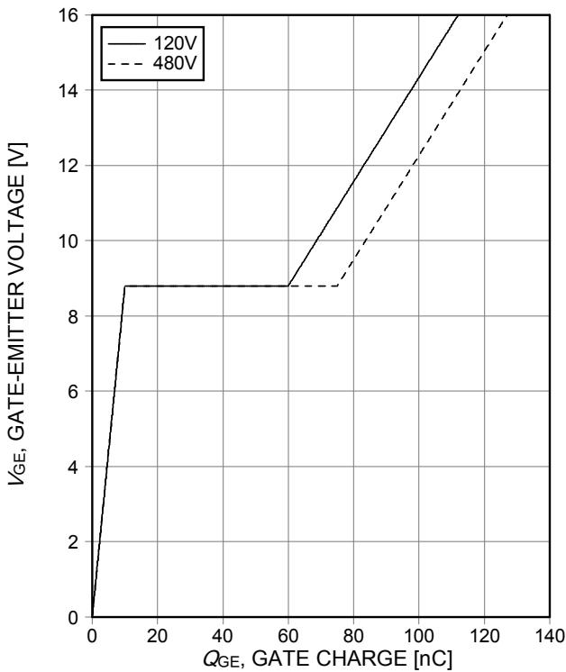
**Figure 17.** Typical gate charge
