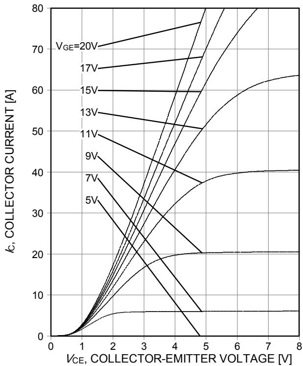
**Figure 6. Typical output characteristic**
