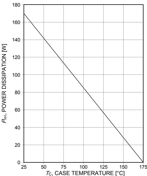
**Figure 3. Power dissipation as a function of case temperature**
