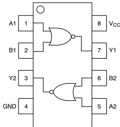
Figure 1. Pinout
