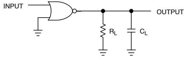
A 1-MHz square input wave is recommended for propagation delay tests.
