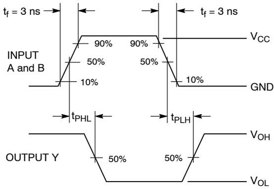
**Figure 3. Switching Waveform**
