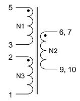
N2 is made of two bifilar windings. Therefore customer has to tie terminals 6+7 and 9+10 on PCB. A general separation of the two windings cannot be guaranteed.
