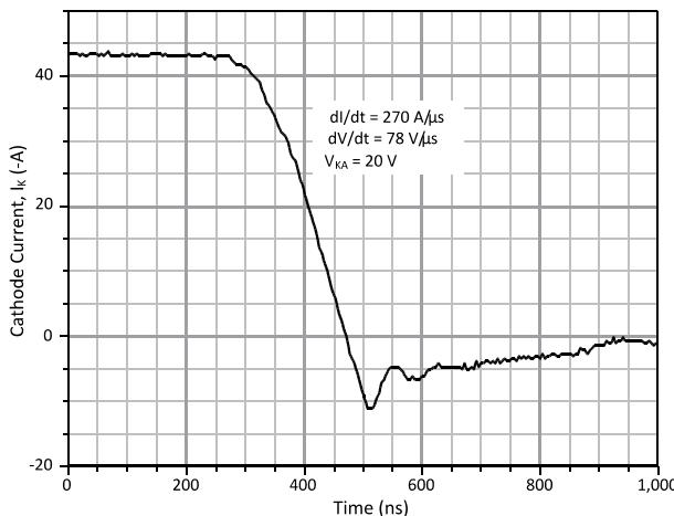
Figure 7: Typical Reverse Recovery Characteristics at 25 °C
