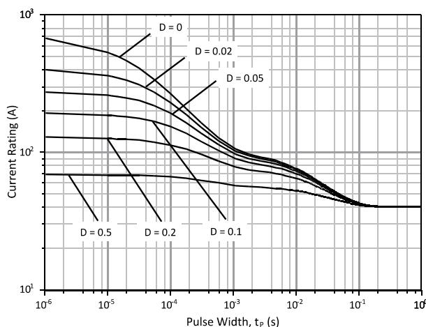
Figure 4: Typical Current Rating versus Pulse Duration Curves
