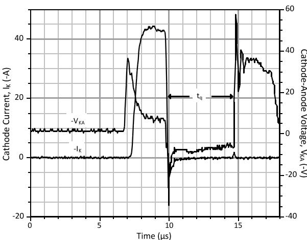
Figure 6: Typical Turn Off Characteristics at  $25^\circ C$
