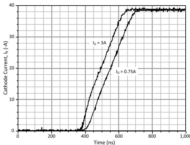
Figure 5: Typical Turn On Characteristics at  $25^\circ C$
