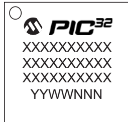
64-Lead TQFP (10x10x1 mm)
