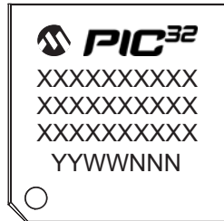
64-Lead TQFP (10x10x1 mm)
