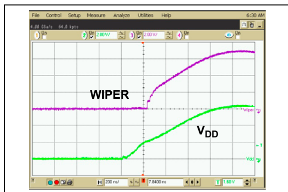
FIGURE 2-15: 2.1 k \Omega – Power-Up Wiper Response Time.
