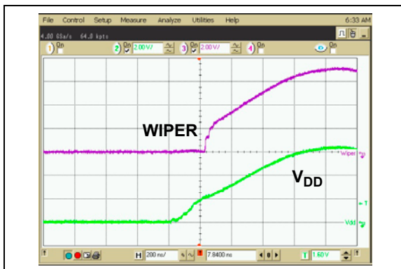
FIGURE 2-52: 50 k \Omega – Power-Up Wiper Response Time.
