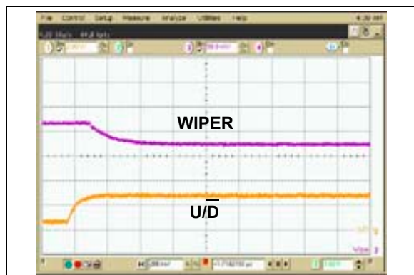
FIGURE 2-13: 2.1 k \Omega – Low-Voltage Decrement Wiper Settling Time ( V_{DD} = 2.7\text{V} ).
