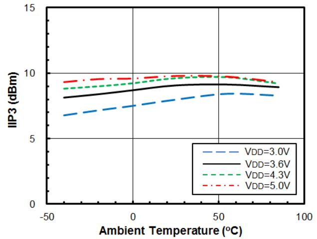
Outband IIP3 vs. Ambient Temperature
