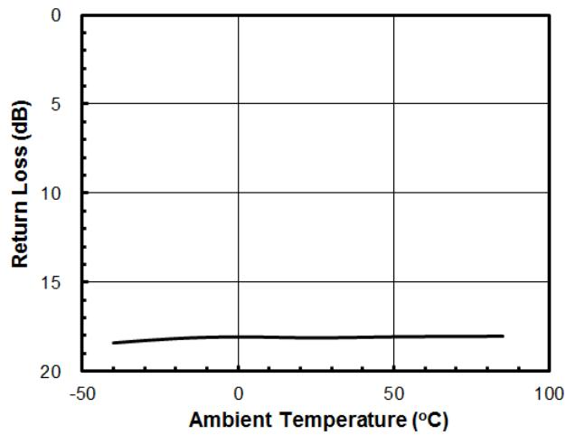
**LNAOUT Port Return Loss vs. Ambient Temperature**
