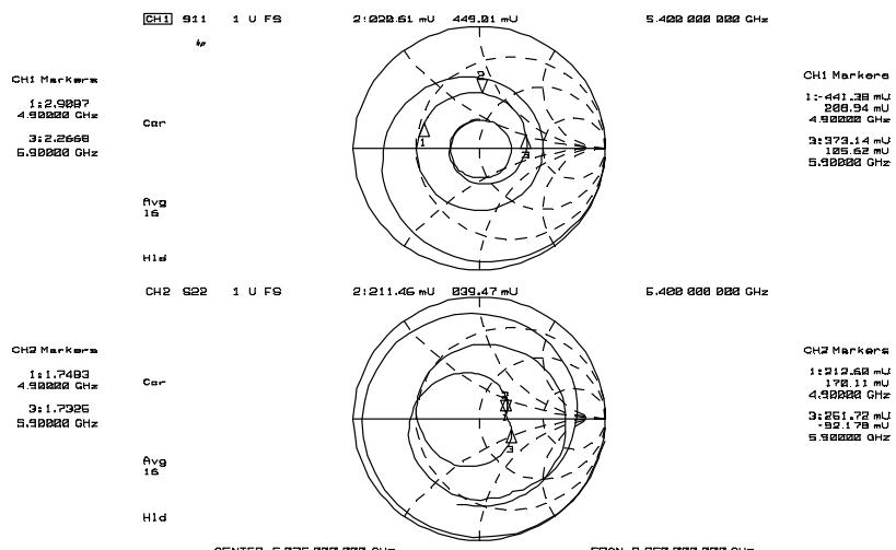
Zin, Zout ( $f=50\text{MHz}$  to  $10\text{GHz}$ )
