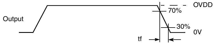
Figure 7. Definition of Timing for Standard and Fast-Mode
