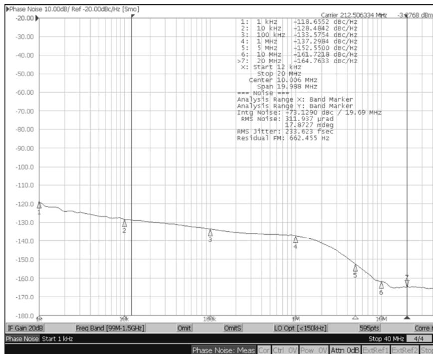
Phase Noise Plot: 212.5MHz, 12kHz – 20MHz 234fS
