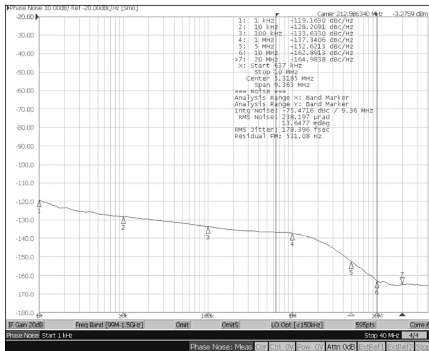
Phase Noise Plot: 212.5MHz, 637kHz – 10MHz 178fS
