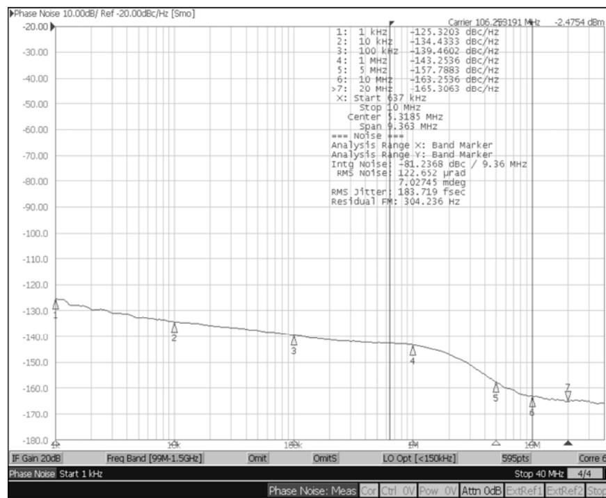
**Phase Noise Plot: 106.25MHz, 637kHz – 10MHz 184fS**
