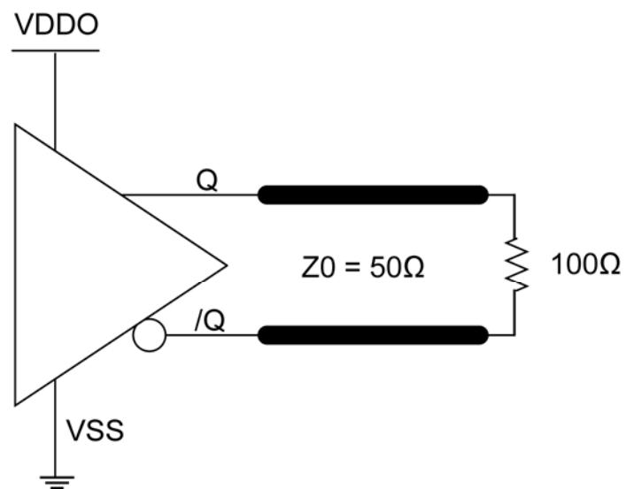
Figure 4. LVDS Output Load and Test Circuit
