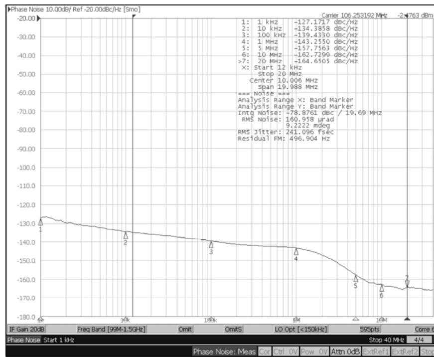
**Phase Noise Plot: 106.25MHz, 12kHz – 20MHz 241fS**
