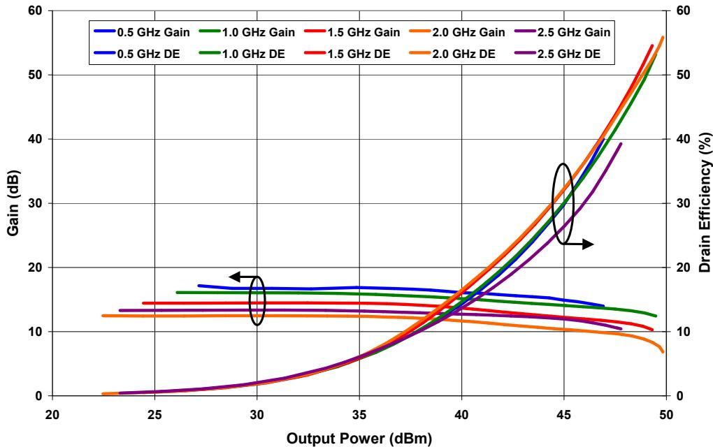
**Output Power and Drain Efficiency vs Frequency of the CGH40090PP measured in Broadband Amplifier Circuit CGH40090PP-TB**
