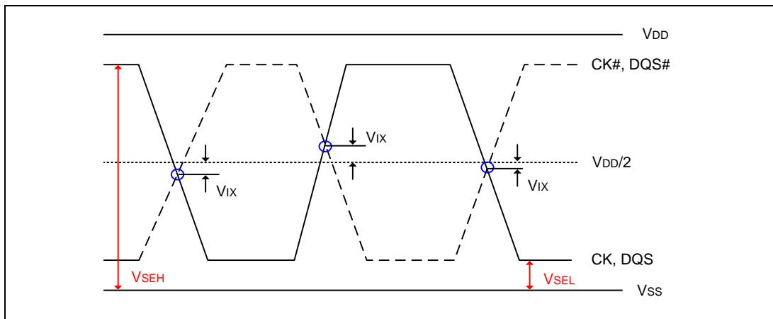
**Figure 92 –  $V_{IX}$  Definition**
