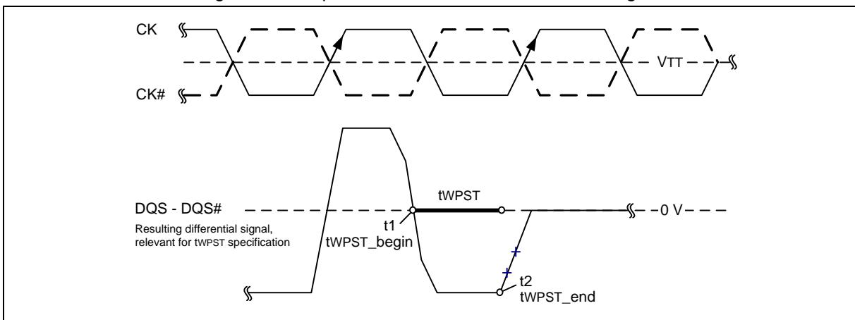
**Figure 42 – Method for calculating tWPST transitions and endpoints**
