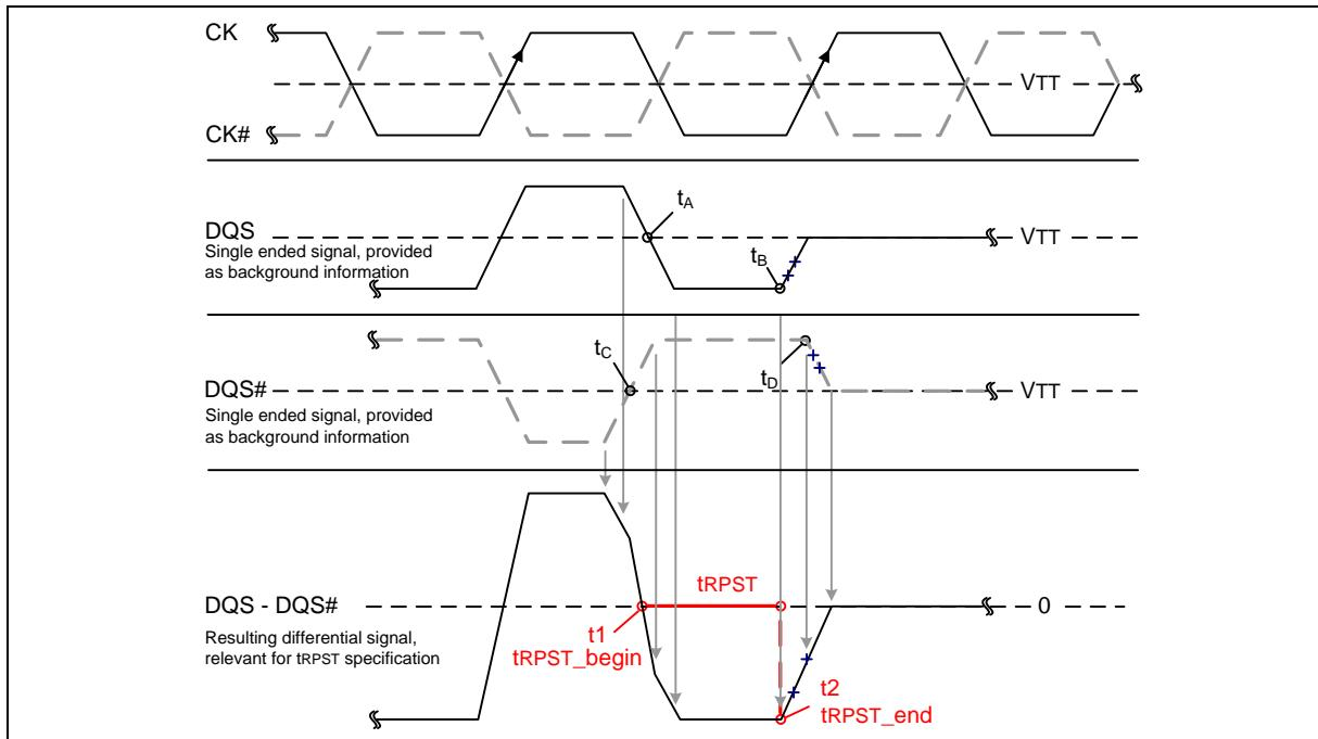
Figure 28 – Method for calculating tRPST transitions and endpoints
