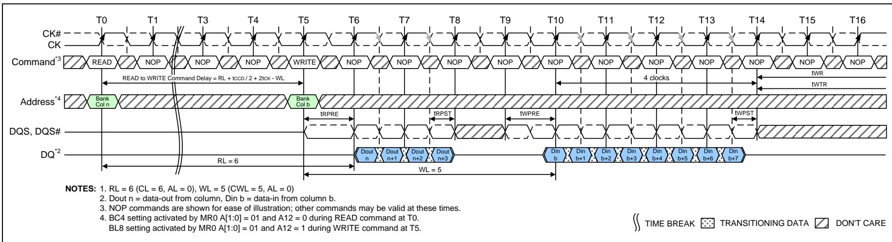
Figure 36 – READ (BC4) to WRITE (BL8) OTF
