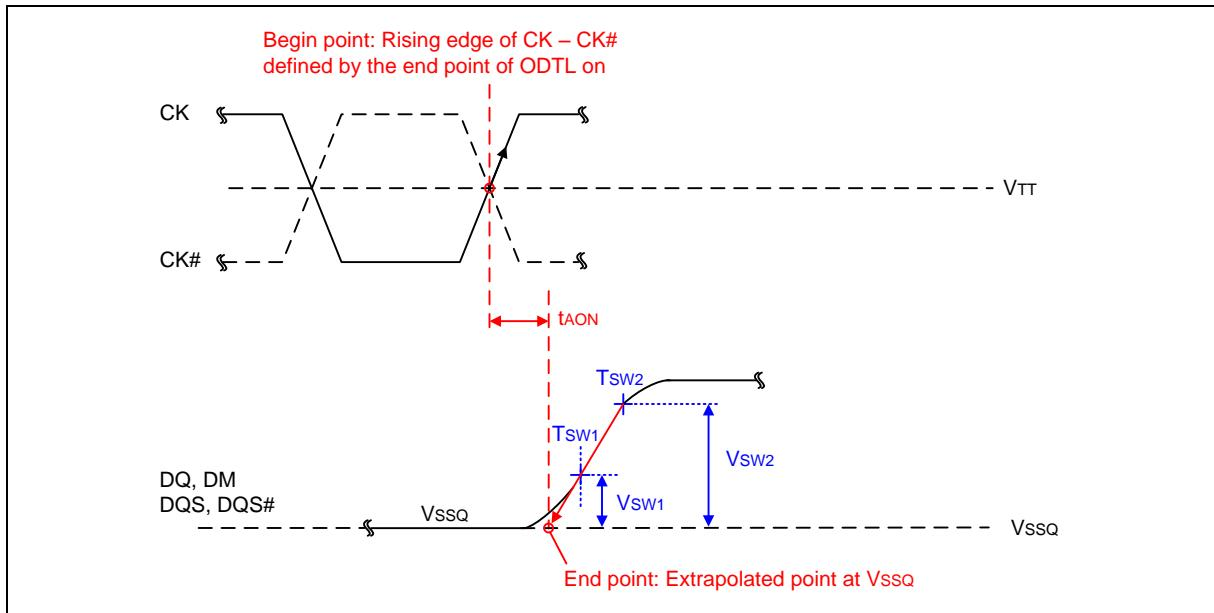
Figure 99 – Definition of t<sub>AON</sub>
