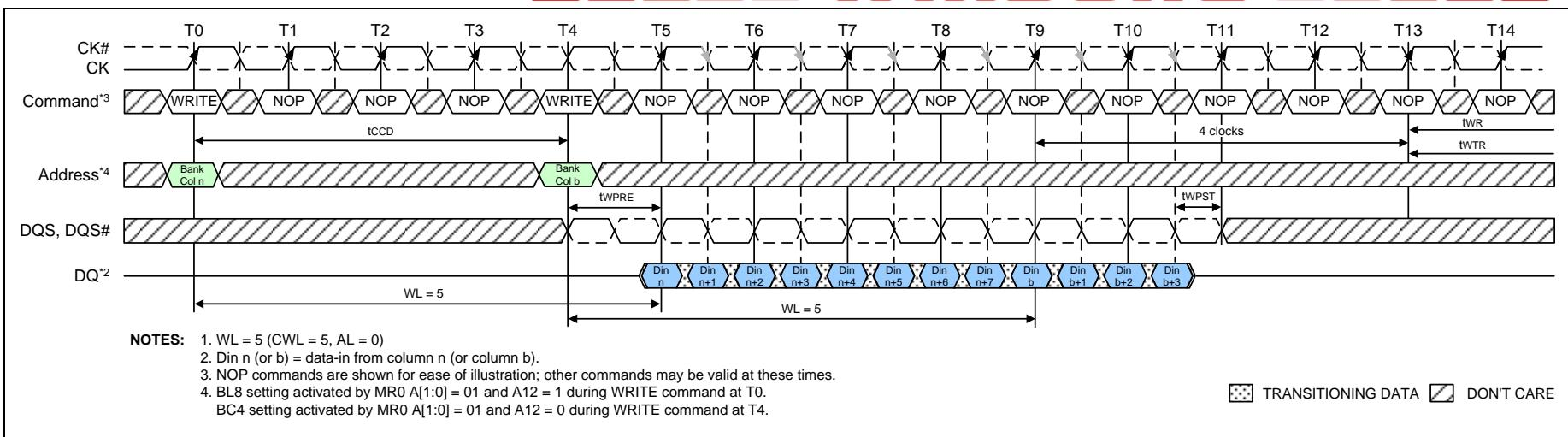
Figure 53 – WRITE (BL8) to WRITE (BC4) OTF
