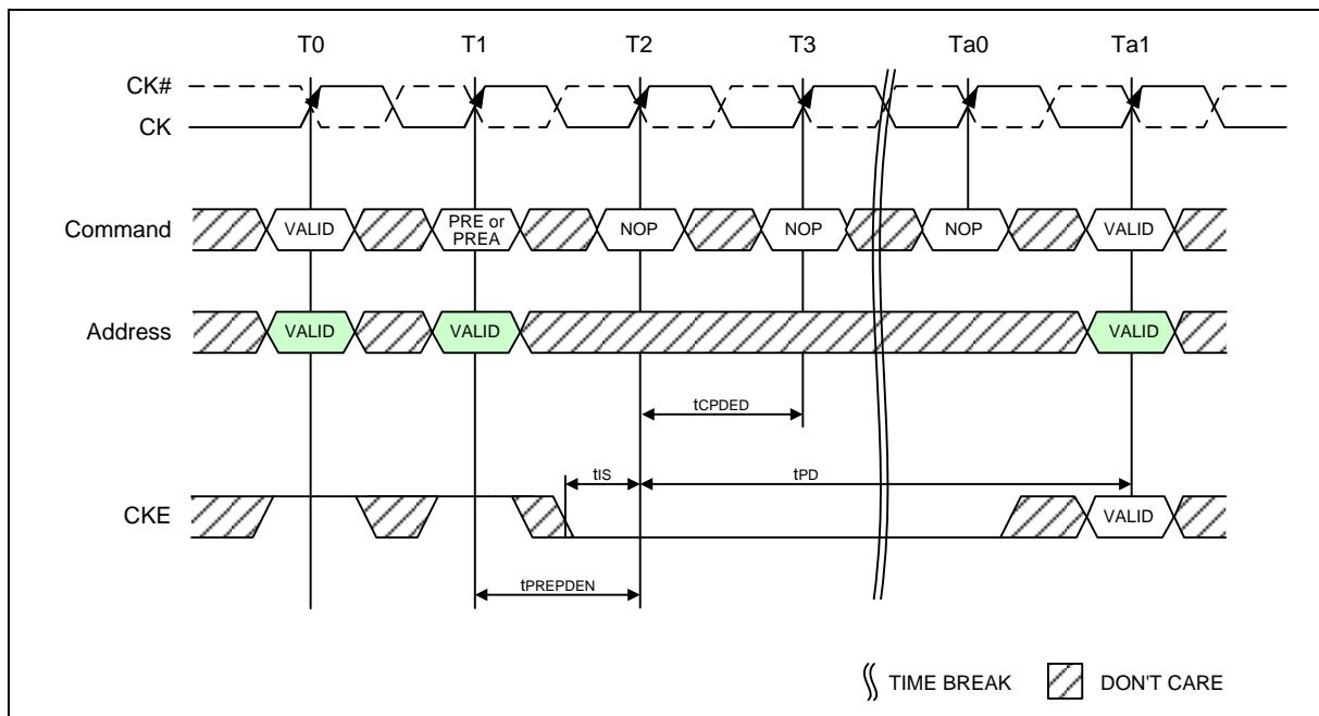
Figure 67 – Precharge / Precharge all Command to Power-Down Entry
