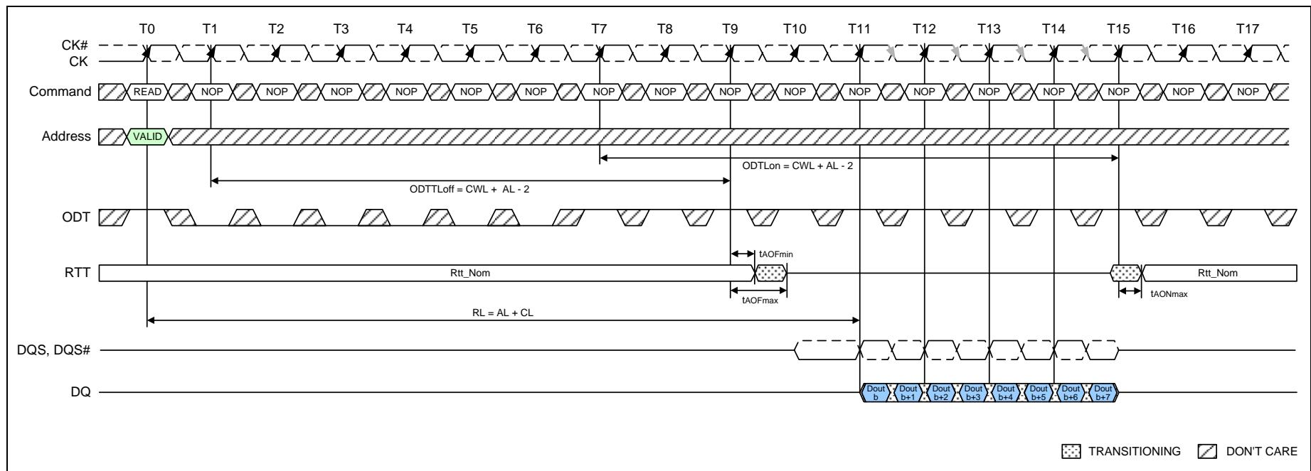
**Figure 76 – ODT must be disabled externally during Reads by driving ODT low.**
