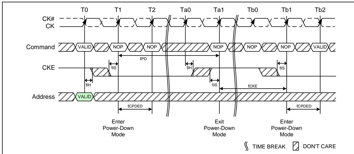
Figure 69 – Power-Down Entry/Exit Clarifications - Case 1
