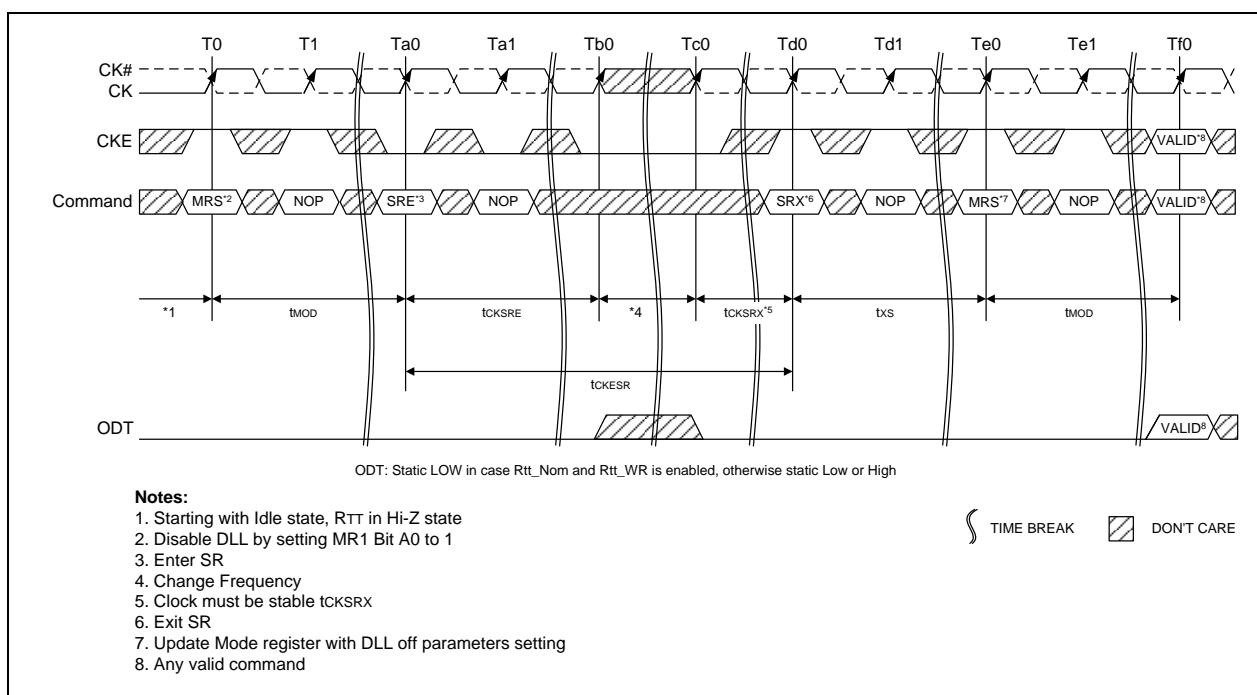
Figure 10 – DLL Switch Sequence from DLL-on to DLL-off
