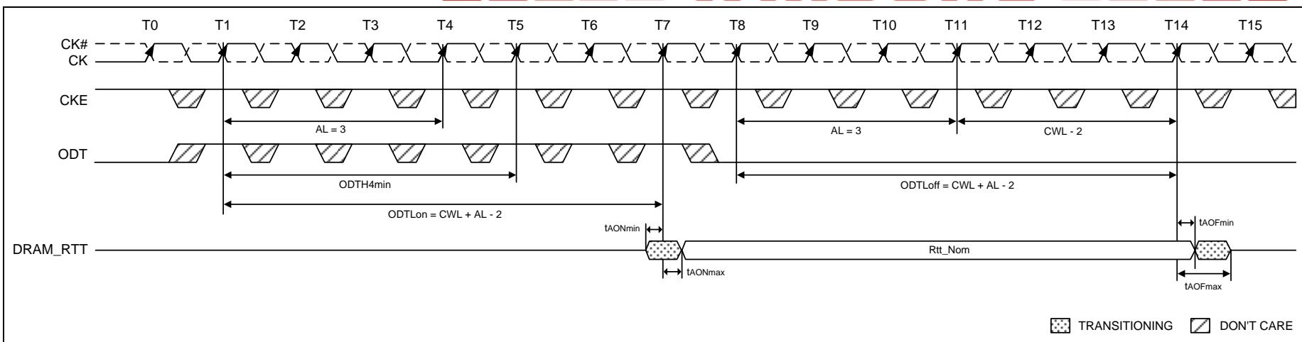
Figure 74 – Synchronous ODT Timing (AL = 3; CWL = 5; ODTLlon = AL + CWL - 2 = 6; ODTloff = AL + CWL - 2 = 6)
