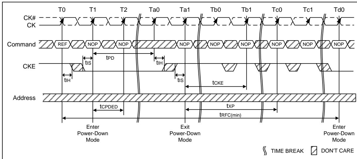
Figure 71 – Power-Down Entry/Exit Clarifications - Case 3
