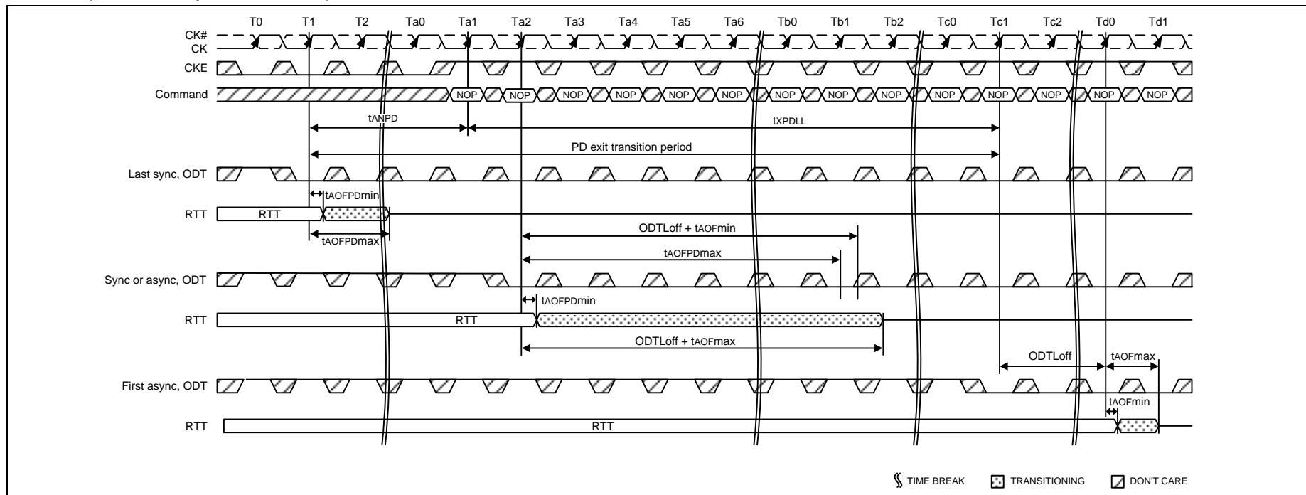
**Figure 85 – Asynchronous to synchronous transition during Precharge Power Down
