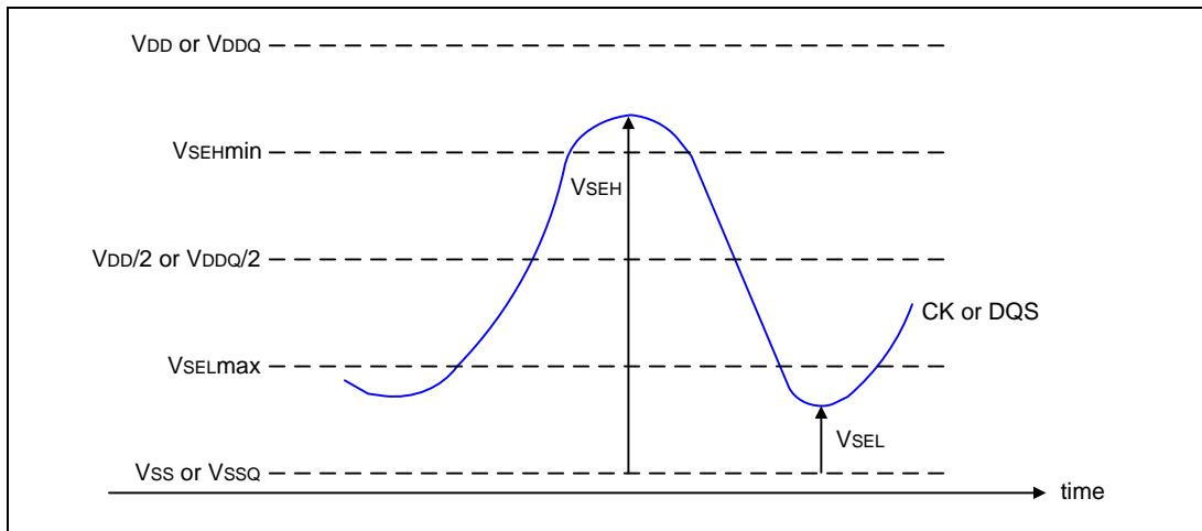
**Figure 91 – Single-ended requirement for differential signals**
