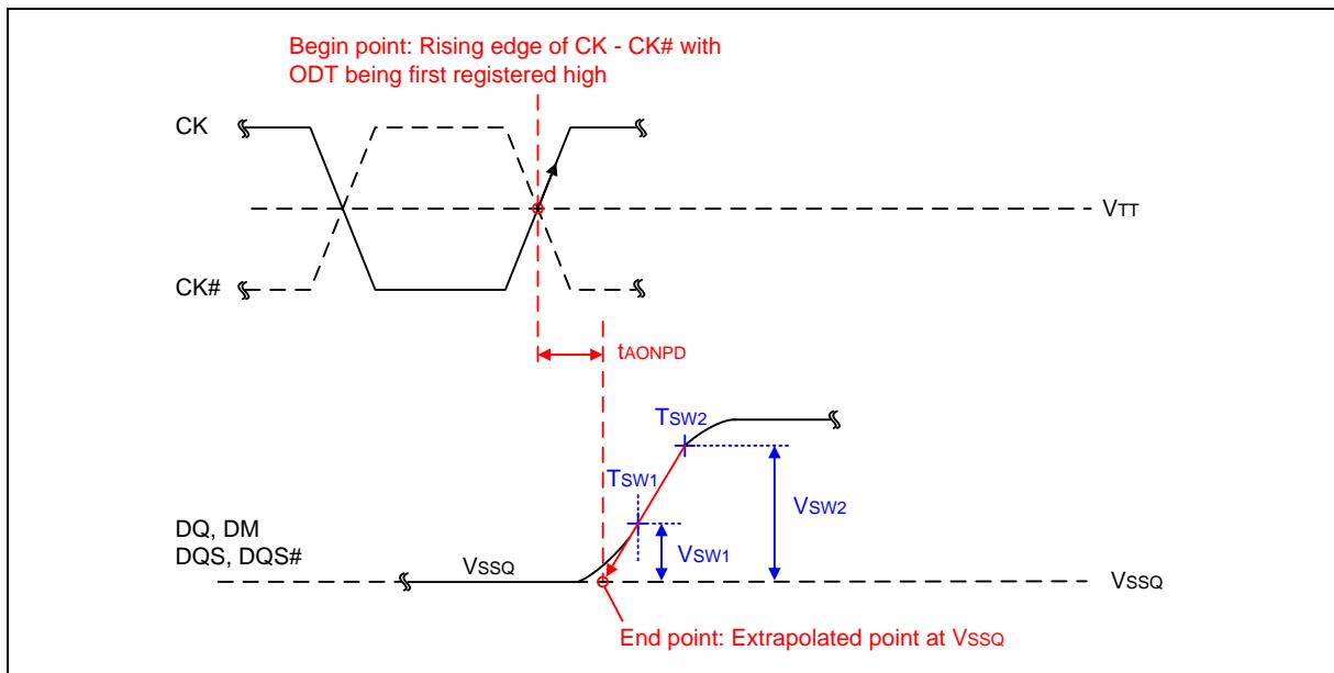
Figure 100 – Definition of t<sub>AONPD</sub>
