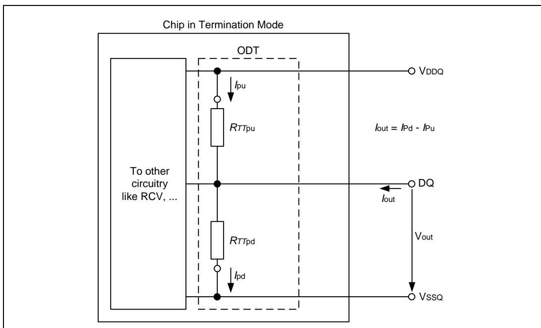
Figure 97 – On-Die Termination: Definition of Voltages and Currents
