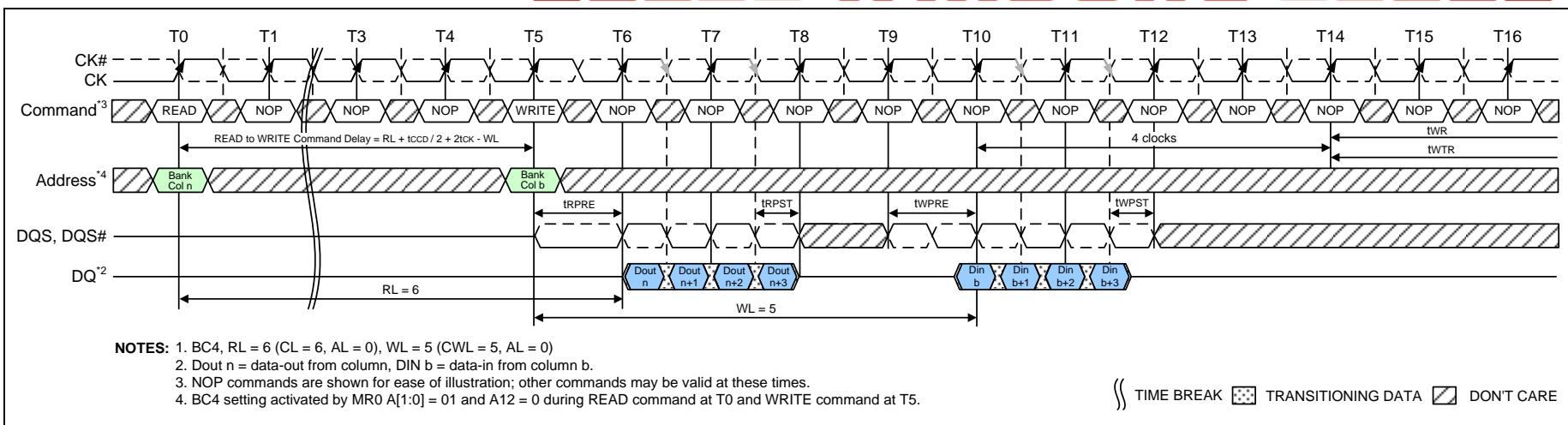
Figure 33 – READ (BC4) to WRITE (BC4) OTF
