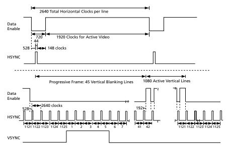
Figure 4-16: H:V:DE Input Timing 1920 x 1080p @ 50 (Format 31)
