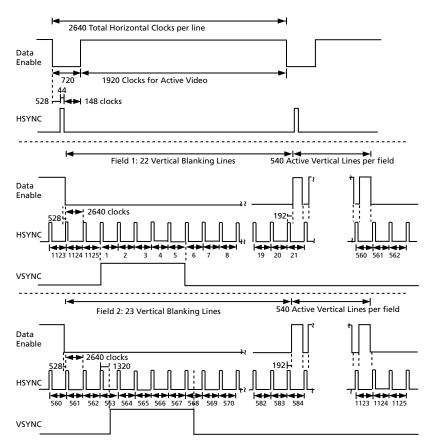
Figure 4-13: H:V:DE Input Timing 1920 x 1080i @ 50 (Format 20)
