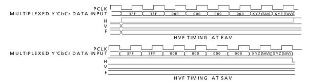
Figure 4-6: H:V:F Input Timing - HD 10-bit Input Mode
