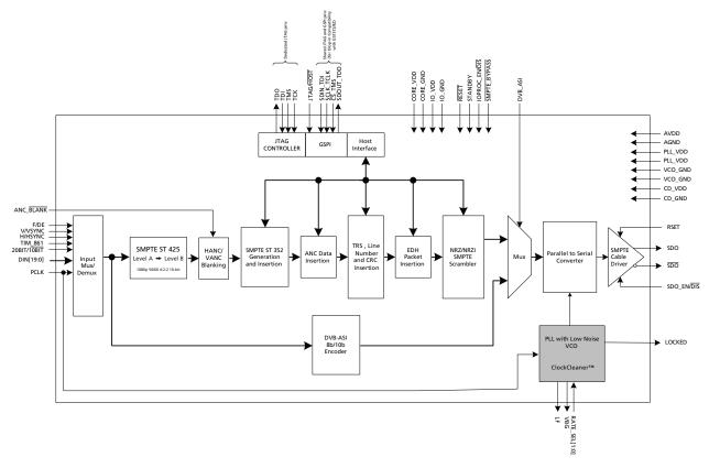
Figure A: GS2962 Functional Block Diagram
