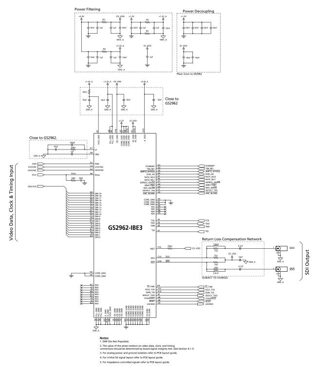
Figure 5-1: Typical Application Circuit
