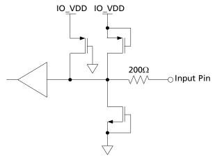
Figure 3-5: Digital Input Pin with weak pull-up - maximum pull-up current <110 $\mu$ A (CS\_TMS, SDO\_EN/DIS, TMS)
