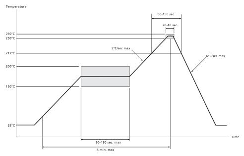
Figure 7-3: Pb-free Solder Reflow Profile
