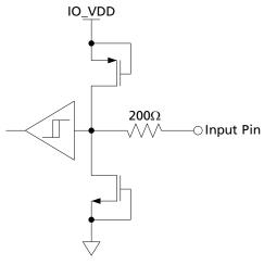
Figure 3-3: Digital Input Pin with Schmitt Trigger (RESET)
