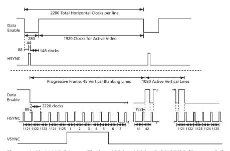
Figure 4-19: H:V:DE Input Timing 1920 x 1080p @ 29.97/30 (Format 34)
