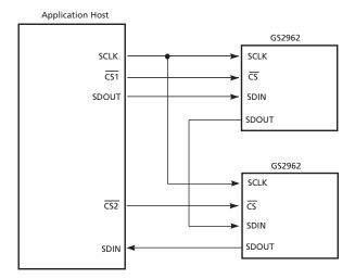
Figure 4-21: GSPI Application Interface Connection
