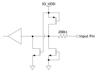
Figure 3-4: Digital Input Pin with weak pull-down - maximum pull-down current <110µA (JTAG/HOST, STANDBY, SCLK\_TCK, SDIN\_TDI, TCK, TDI)
