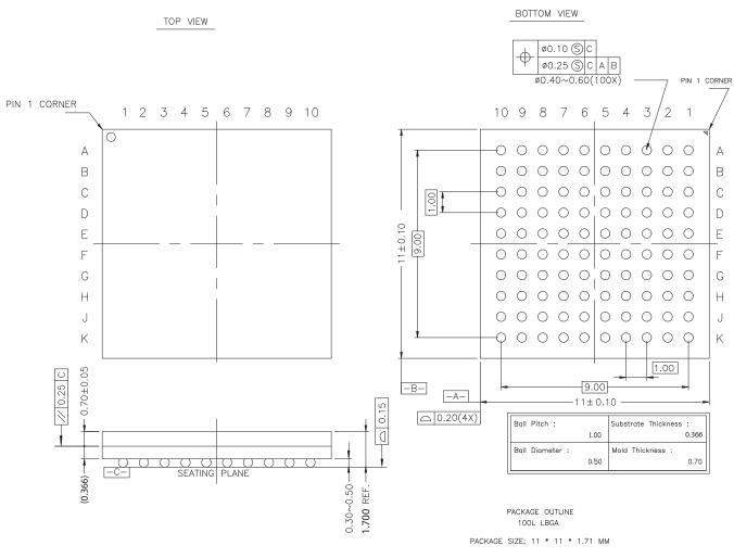
\* THE BALL DIAMETER, BALL PITCH, STAND-OFF & PACKAGE THICKNESS ARE DIFFERENT FROM JEDEC SPEC M0192 (LOW PROFILE BGA FAMILY)
