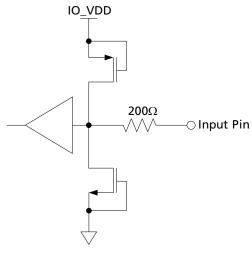
Figure 3-2: Digital Input Pin (20bit/10bit, ANC\_BLANK, DETECT\_TRS, DVB\_ASI, RATE\_SEL0, SMPTE\_BYPASS, RATE\_SEL1, TIM\_861, F/DE, H/HSYNC, PCLK, V/VSYNC)
