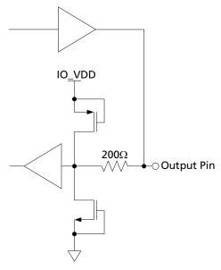
Figure 3-7: Bidirectional Digital Input/Output Pin with programmable drive strength. These pins are configured to output at all times except in reset mode. (LOCKED, SDOUT\_TDO, TDO)
