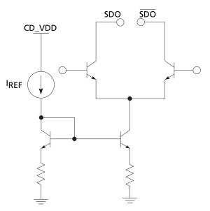
Figure 3-1: Differential Output Stage (SDO/SDO)
