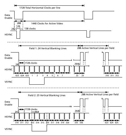
Figure 4-14: H:V:DE Input Timing 720 (1440) x 576 @ 50 (Format 21&22)
