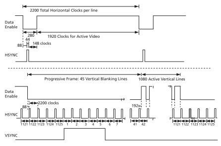
Figure 4-15: H:V:DE Input Timing 1920 x 1080p @ 59.94/60 (Format 16)
