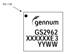
XXXXXX - Last 6 digits (excluding decimal) of SAP Batch Assembly (FIN) as listed on Packing Slip.
