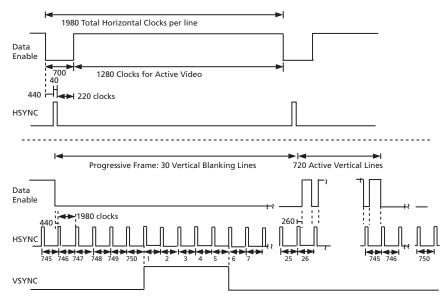
Figure 4-12: H:V:DE Input Timing 1280 x 720p @ 50 (Format 19)
