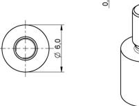
Technical Tolerances according to DIN ISO 2768m In tape & reel packaging a cap is fixed to the product to realize automatic assembly
