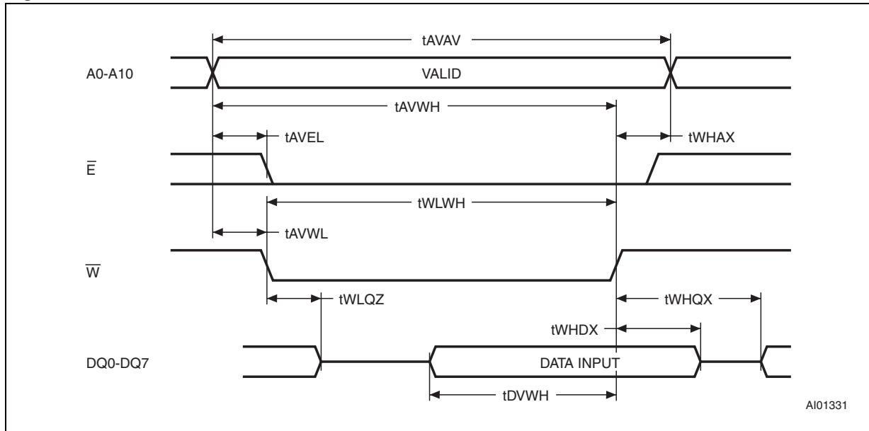
**Figure 6.** Chip enable controlled, WRITE AC waveforms
