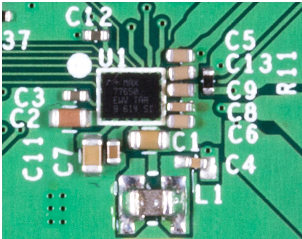
Figure 5. MAX77650 Top View Main Components
