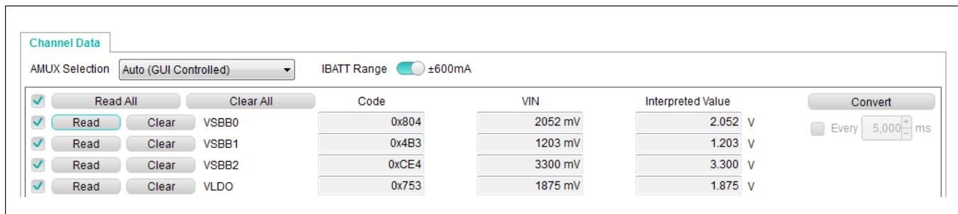
Figure 6. Quick Start: Regulator Check with the ADC
