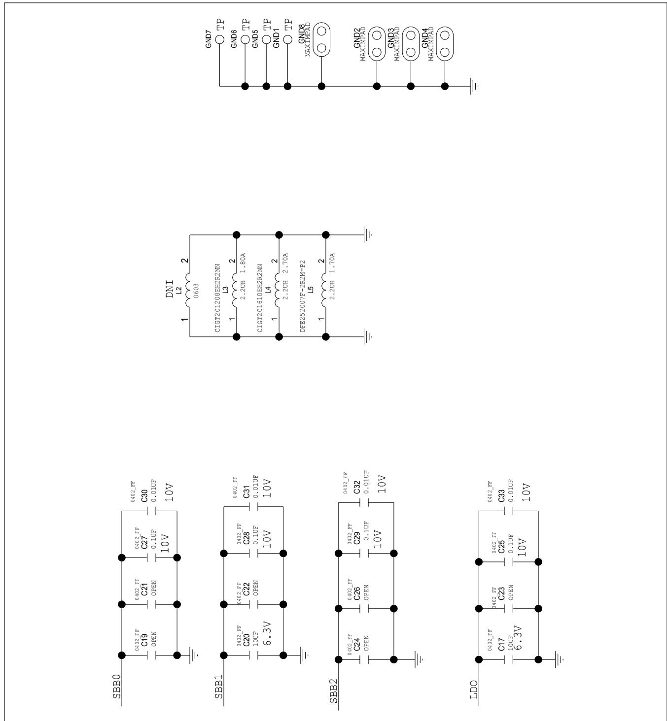
Figure 11. MAX77650/MAX77651 EV Kit Schematic (3 of 6)
