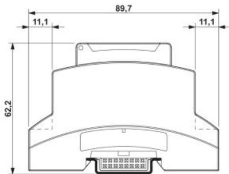
The dimensional drawing shows the item with the lower part of the housing and the housing cover
