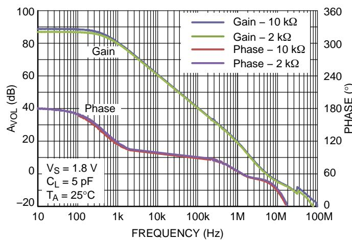
**Figure 11. Open Loop Gain and Phase vs. Frequency @  $V_S = 1.8$  V**
