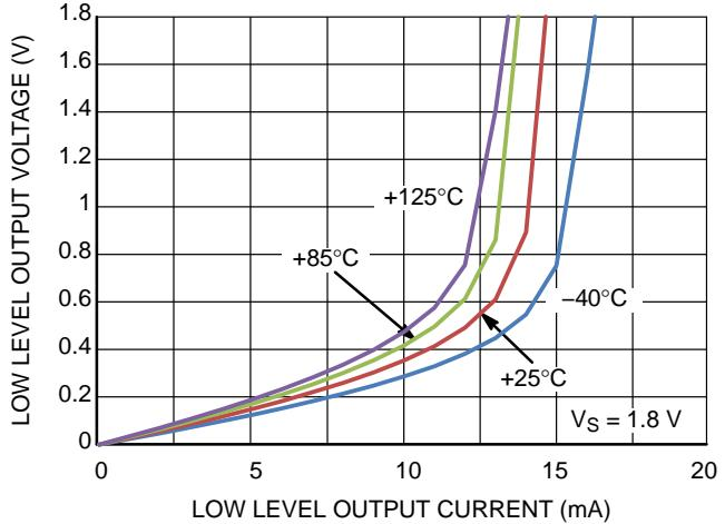
Figure 5. Low Level Output Voltage vs. Output Current @  $V_S = 1.8\text{ V}$
