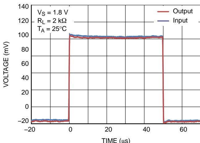
**Figure 15. Non-Inverting Small Signal Transient Response**
