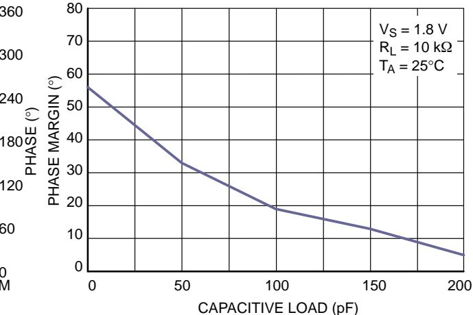
**Figure 13. Phase Margin vs. Capacitive Load**
