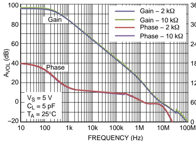
**Figure 12. Open Loop Gain and Phase vs. Frequency @  $V_S = 5$  V**
