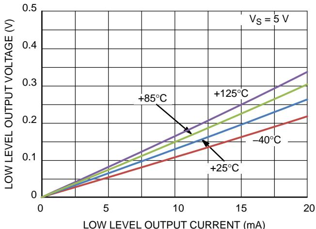
Figure 6. Low Level Output Voltage vs. Output Current @  $V_S = 5\text{ V}$
