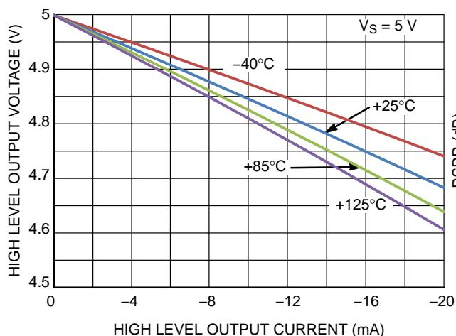
**Figure 8. High Level Output Voltage vs. Output Current @  $V_S = 5$  V**
