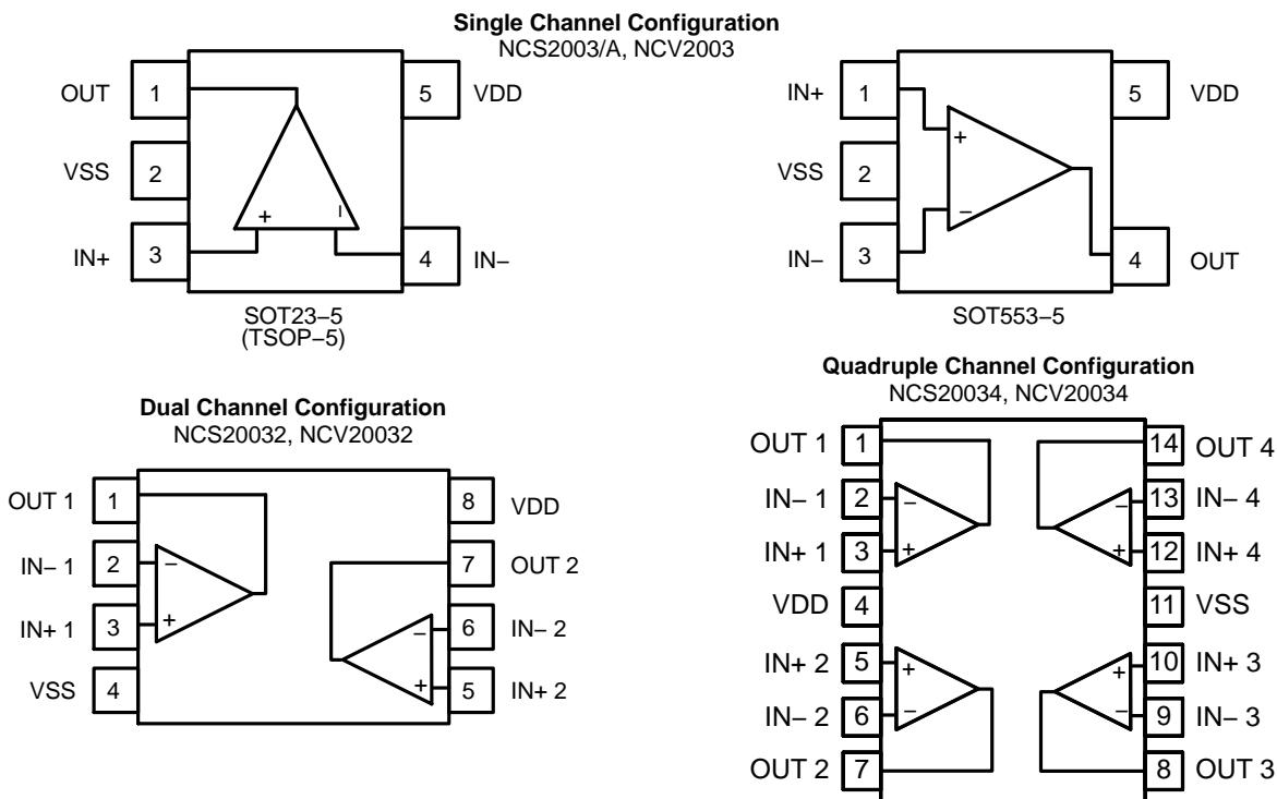
Figure 1. Pin Connections
