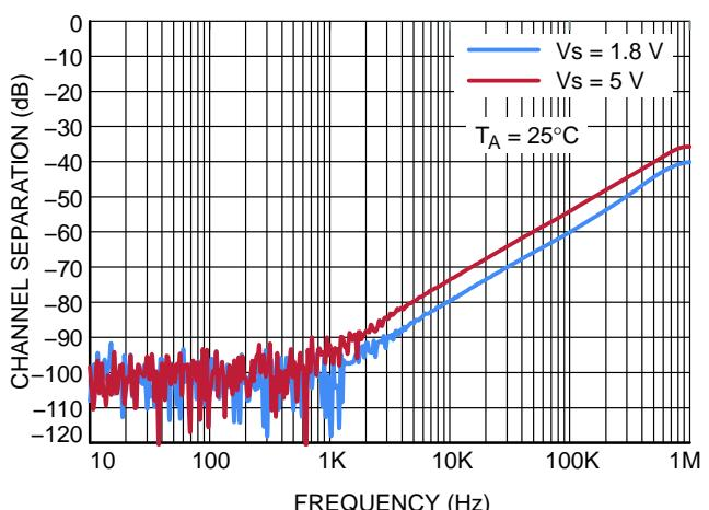
Figure 25. Channel Separation
